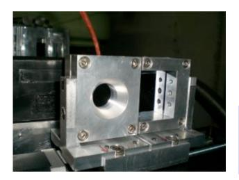
Quasi-Mosaic Crystals have been fabricated in PNPI (Gatchina, Russia) Crystal plate sizes: ~ 1 × 30 × 55 mm<sup>3</sup> critical angle for 400 GeV/c protons  $\theta_c \approx 10 \mu rad$
