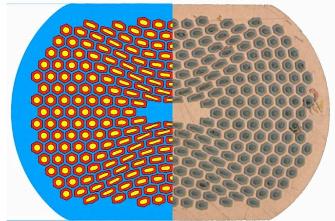
Side-by-side comparisons of computed and observed deformations of un-reacted "internal tin" (left) and "PIT" (right) wires
