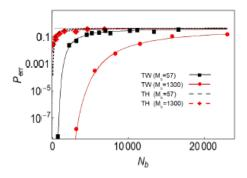
**Fig. 1:** Error probability of discriminating if the target is present or not in function of the number photons  $N_b$  of the background. TW and TH stand for TWin beams and THermal split beams respectively, while Mb is the number of independent modes of the multi-thermal background
