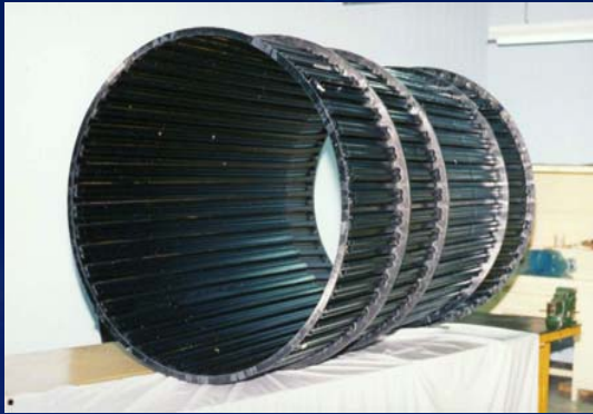
Structure Central Tube
