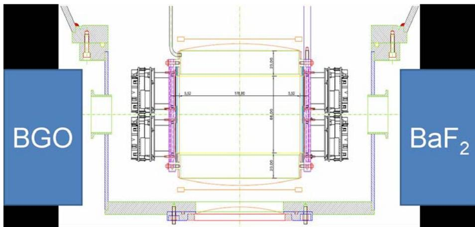
Fig. 15. Possible placement of gamma rays detectors around the target cell (outside the vacuum jacket)
