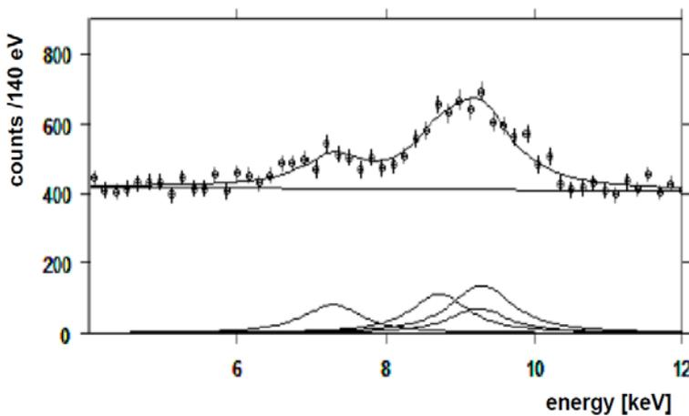
Fig. 7: MC simulation of the expected  $Kd$  spectrum for the SIDDHARTA-2 upgrade taking the SIDDHARTA measurement into account. For an integrated luminosity of  $600 \text{ pb}^{-1}$  the shift could be extracted with about 10%.
