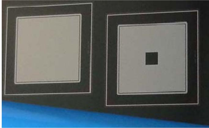
Fig. 13: Picture of two prototype Si-PIN diode cells with a size of 6mm x 6 mm
