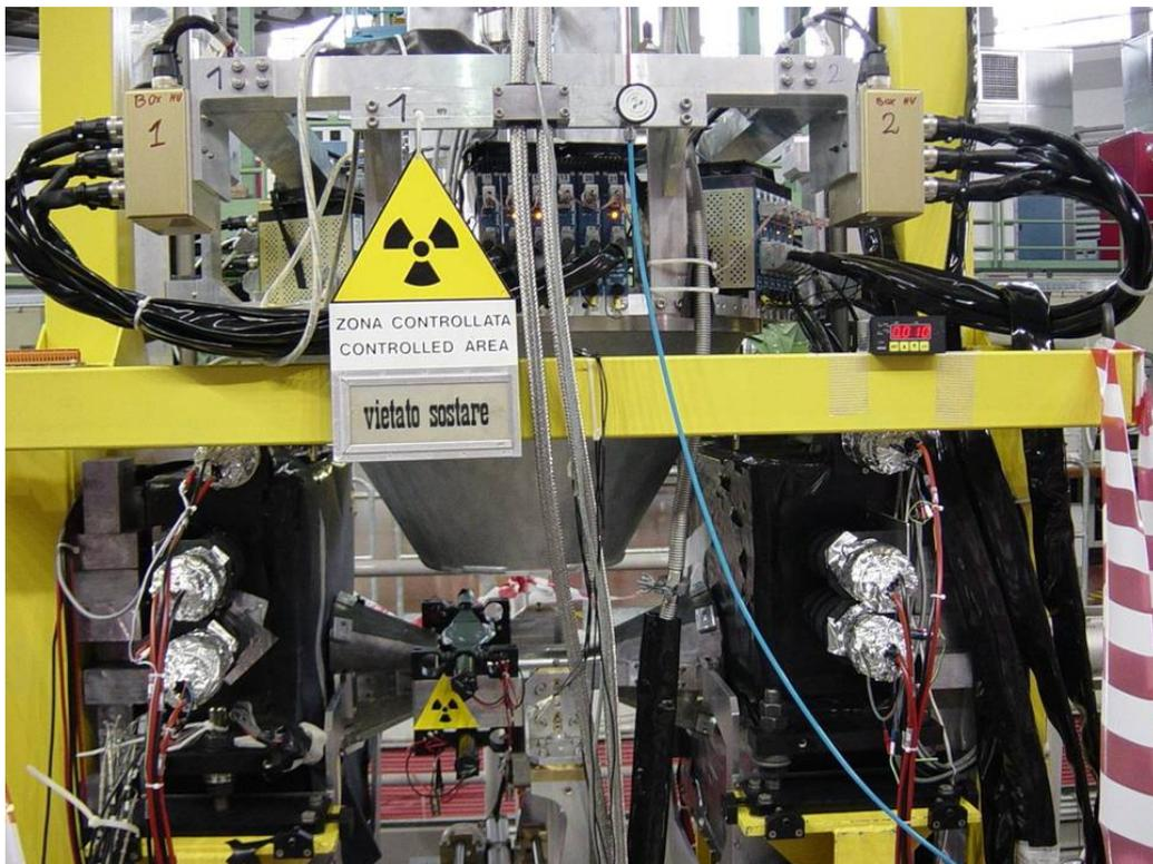
*Fig. 1 The SIDDHARTA setup installed on the DAΦNE Accelerator*
