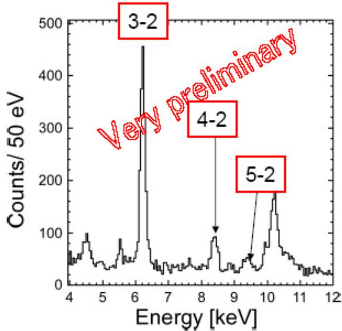
Fig. 5: Kaonic Helium3 preliminary spectrum where the transitions to the 2p level are clearly identified.
