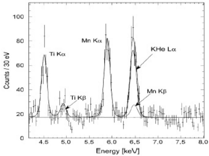
Fig. 3: Energy spectrum of the kaonic 4He X-rays. The kaonic 4He La line is seen at 6.4 KeV.
