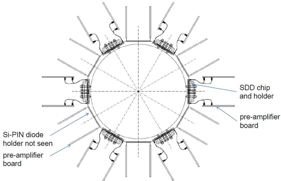
*Fig. 14: Schematic of the SIDDHARTA-2 setup with a combined arrangement of SDDs and Si-PINs in SIDDHARTA-2 (sid-view and top-view). Due to a new design of the Si-PIN we will achieve a factor of 3 larger active to total area than with SDDs.*
