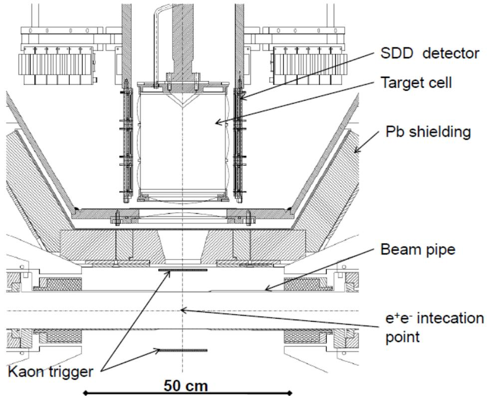
Fig. 2 Sketch of the SIDDHARTA setup; the target cell is surrounded by SDD detectors, placed within a vacuum chamber, surrounded by a lead shield.
