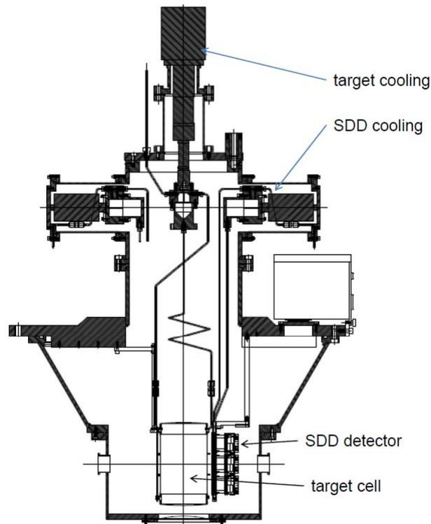
*Fig. 11: The SIDDHARTA2 setup – showing the new liquid hydrogen and liquid argon closed cooling systems to be used for target and SDDs; strongly reducing the material budget on top of the target cell.*
