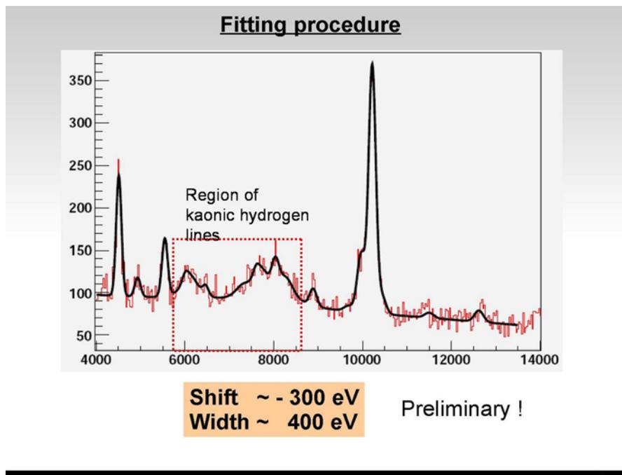
Fig. 4: Kaonic hydrogen preliminary spectrum
