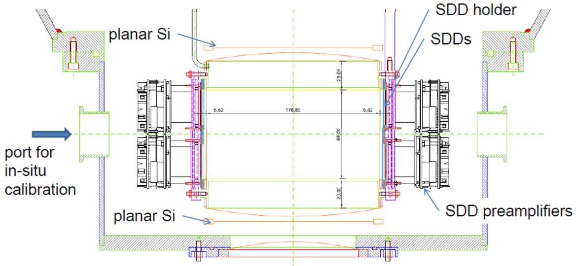
*Fig. 10: The new vacuum jacket, target cell and SDD/Si-PIN arrangement for SIDDHARTA-2; side view.*
