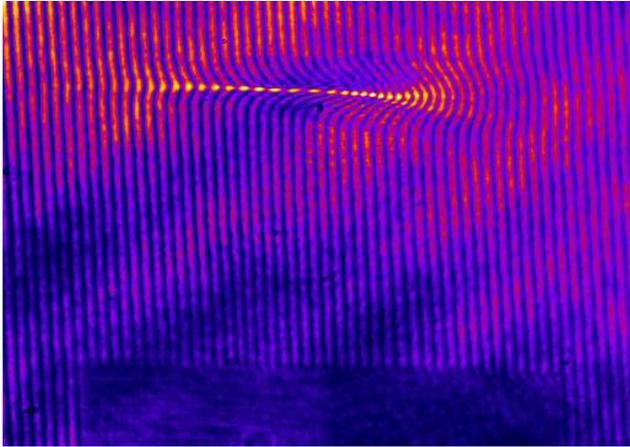
MachZender interferometer to measure the plasma density.
