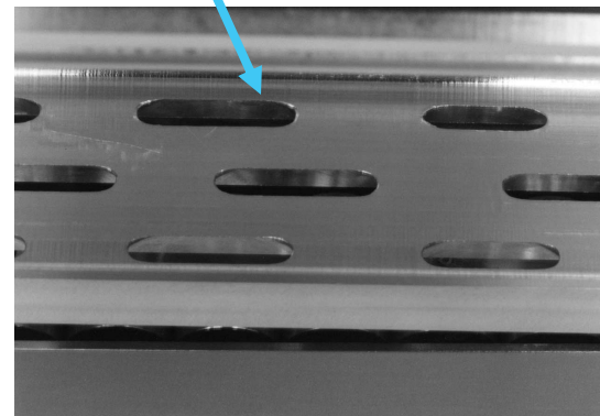
Asymmetric slots for vacuum pumping Avoid overlap with beam spectrum
