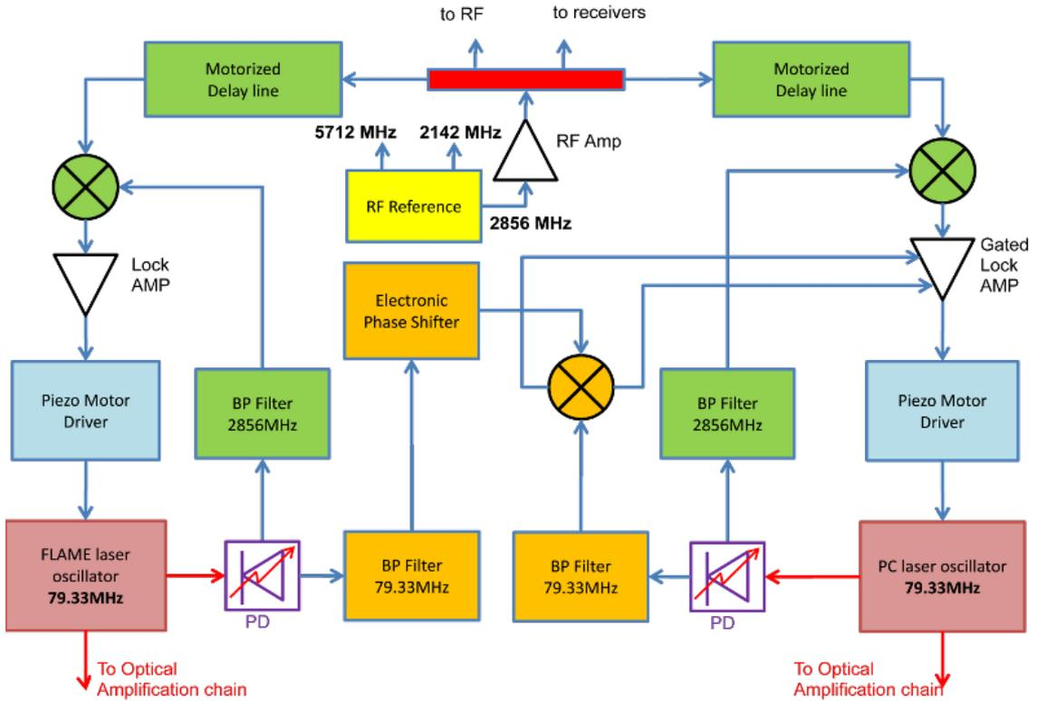
Figure 1: SPARC Lab electrical synchronization system schematics
