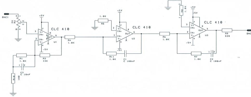
Figure 6: Error amplifier providing a triple integrator frequency response (PLL3)
