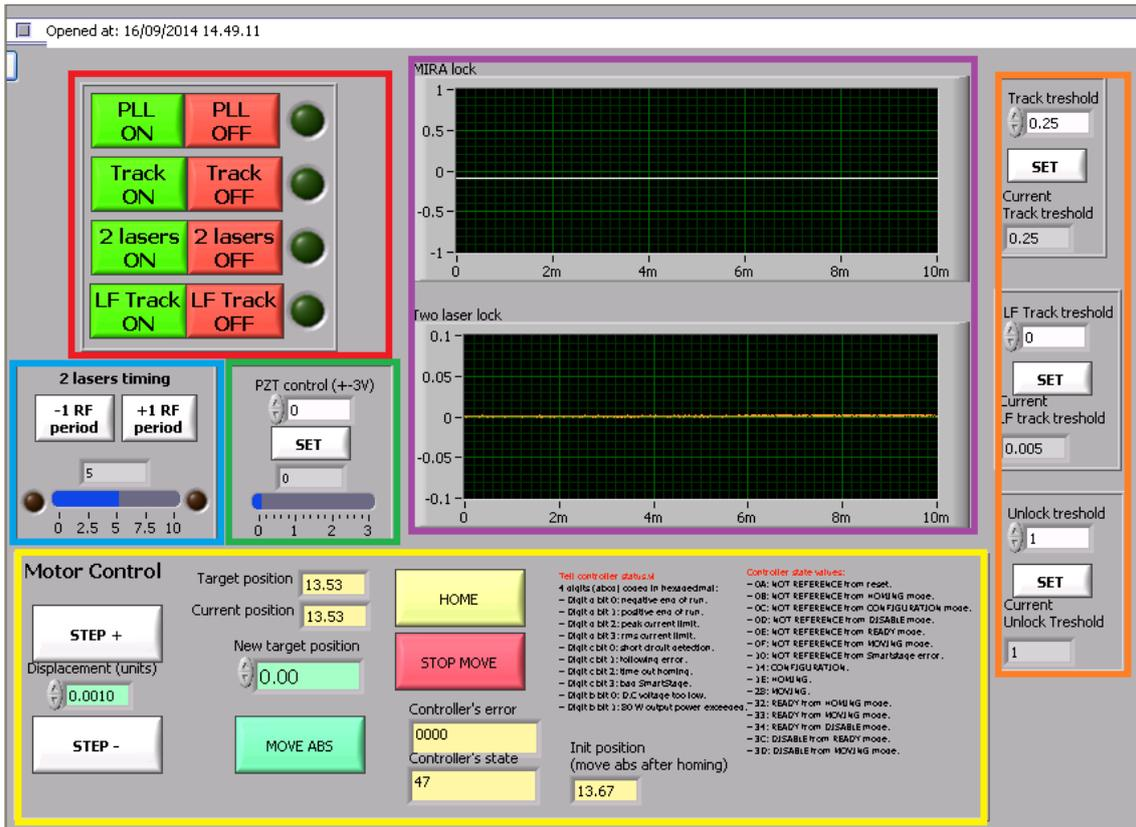
Figure 10: The control room GUI for controlling the new SPARC\_LAB locking features
