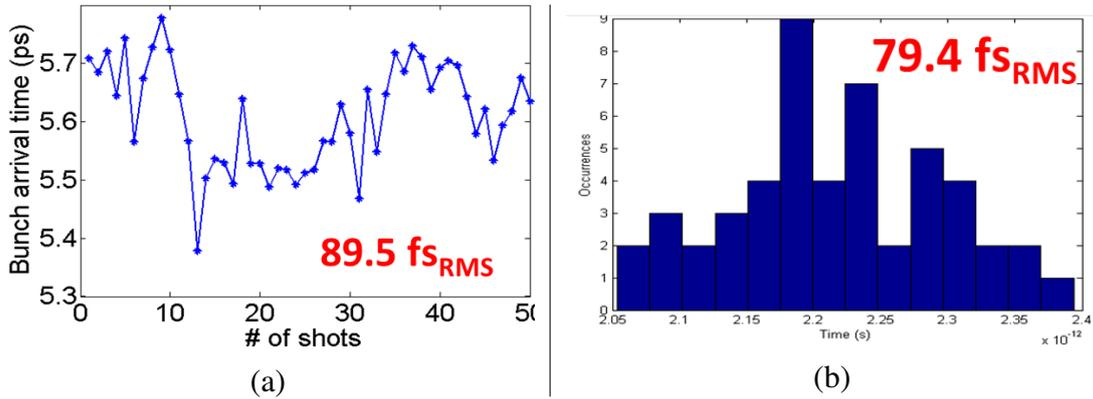
Figure 8: Diagnostics on the electron beam time jitter
