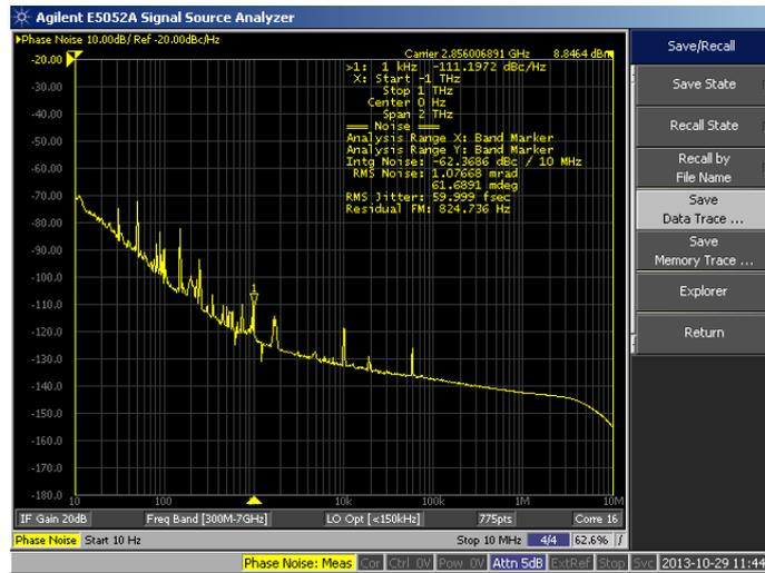
Figure 2: SSB phase noise spectrum of the SPARC LAB RMO
