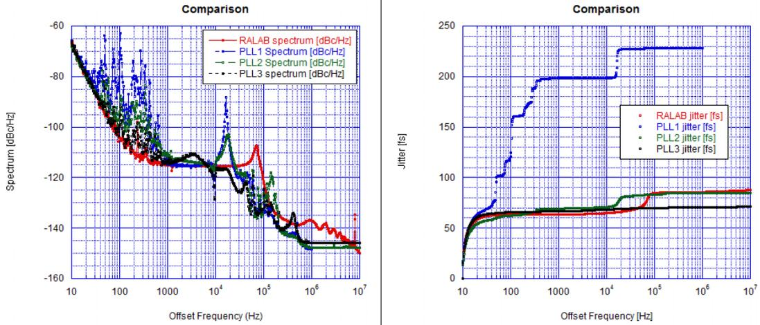
Figure 5: SSB phase noise spectrum and integrated jitter of the MIRA laser oscillator with different PLLs
