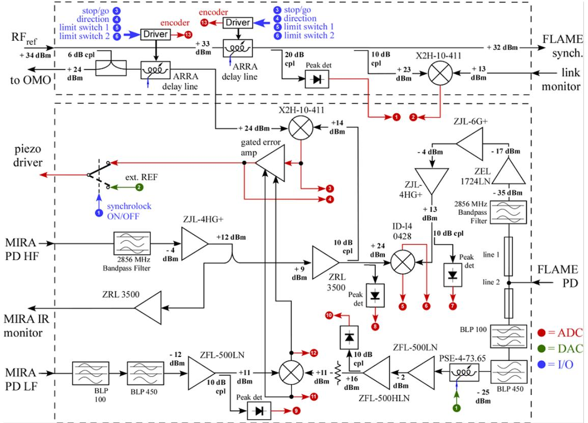
Figure 7: Block diagram of the MIRA-FLAME synchronization system
