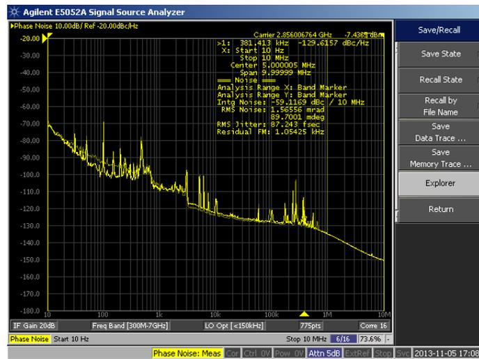
Figure 4: SSB phase noise spectrum of the FLAME oscillator locked to the RMO signal
