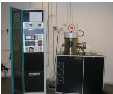
Figure 1: the RF magnetron sputtering apparatus from IONVAC PROCESS srl.
