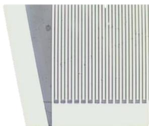
Figure 2: interdigitated Mo electrode geometry obtained by lift off process
