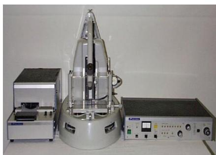
Figure 3: The mechanical profilometer used to measure the thickness of the thin Mo films grown on the reference samples (courtesy of IDASC-CNR).
