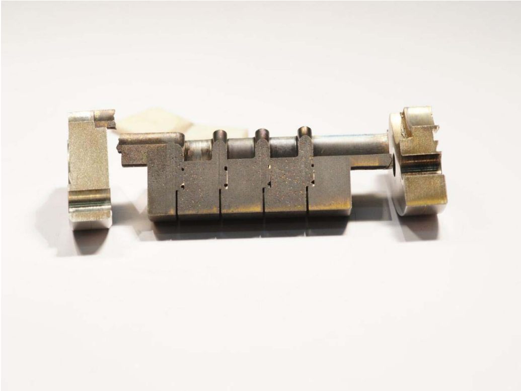
Fig 2 When one of the sections was cut again (also by EDM) both flanges on one of the pieces (a 1/4 section of the whole) detached as shown
