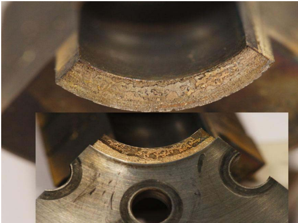
Fig 2 When one of the sections was cut again (also by EDM) both flanges on one of the pieces (a 1/4 section of the whole) detached as shown
