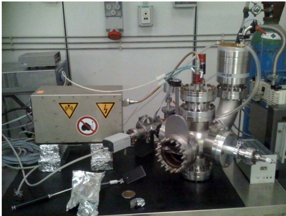
Fig. 1 Experimental set up for the RF Magnetron Sputtering .
