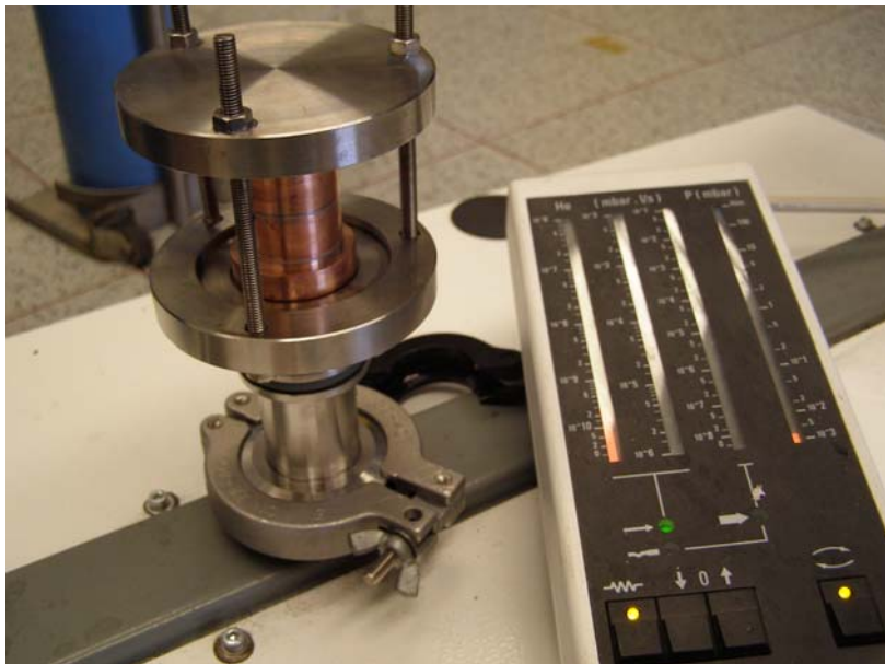
Fig 2 : A Cu OFHC structure under vacuum leak test.
