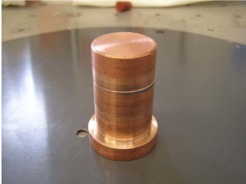
Fig 1: Soft brazed 3 cells Cu prototype.
