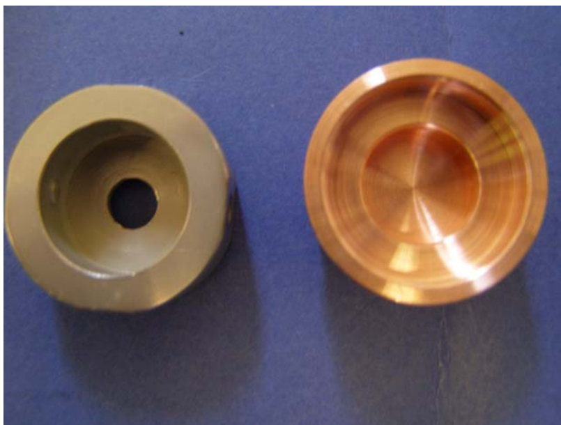
Fig 3 : The Ag/Sn alloy deposited on copper object by sputtering technique.
