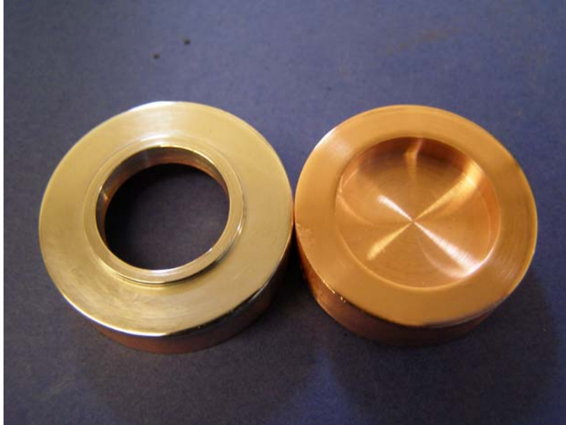
Fig 4 : Electrolytically deposited Sn on copper object
