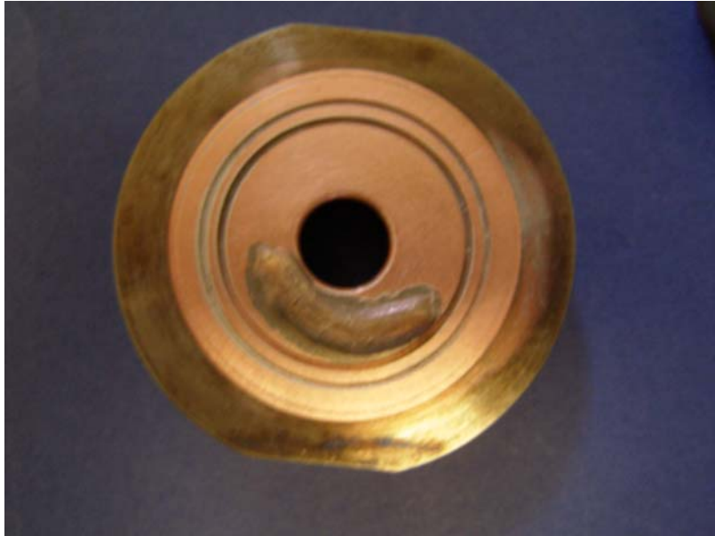
Fig 2 : Copper electrolessly deposited on the molybdenum cell with the Cusil alloy after thermal treatment .
