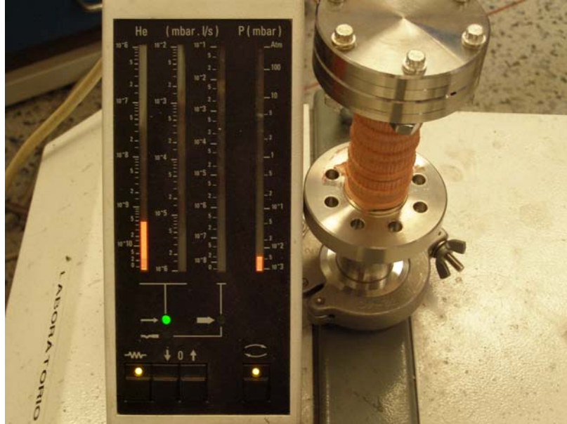
Fig 6 : A 3 cell Cu OFHC structure, encapsulated by galvanoplastic procedure under vacuum leak test.
