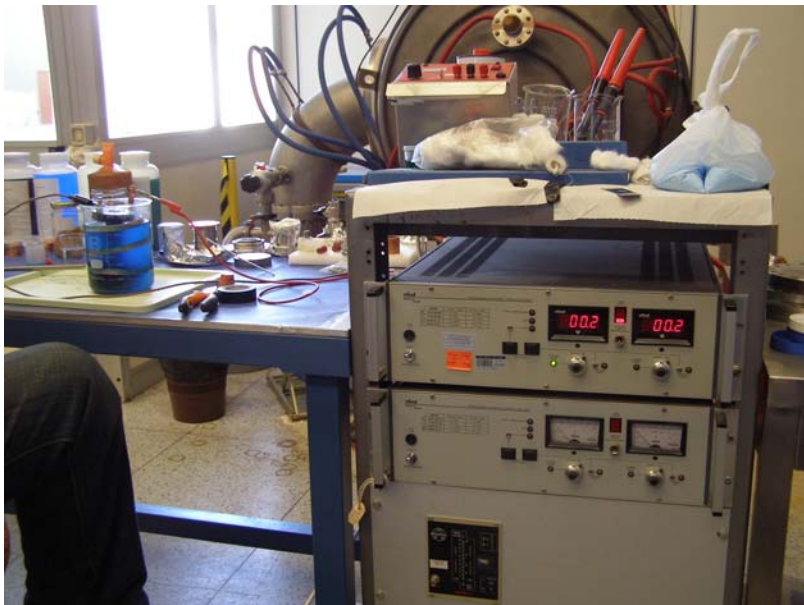
Fig 5 The encapsulation procedure for a three cells , Cu OFHC structure.
