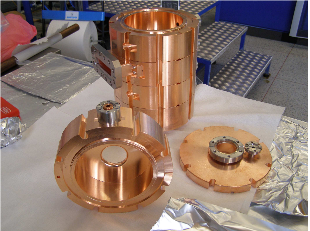
Fig 7 Some parts of the RF deflector during brazing procedure.
