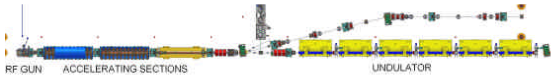
FIG. 1: Layout of the SPARC linear accelerator
