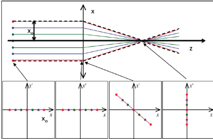
Fig. 1 Particle trajectories and phase space evolution of a laminar beam
