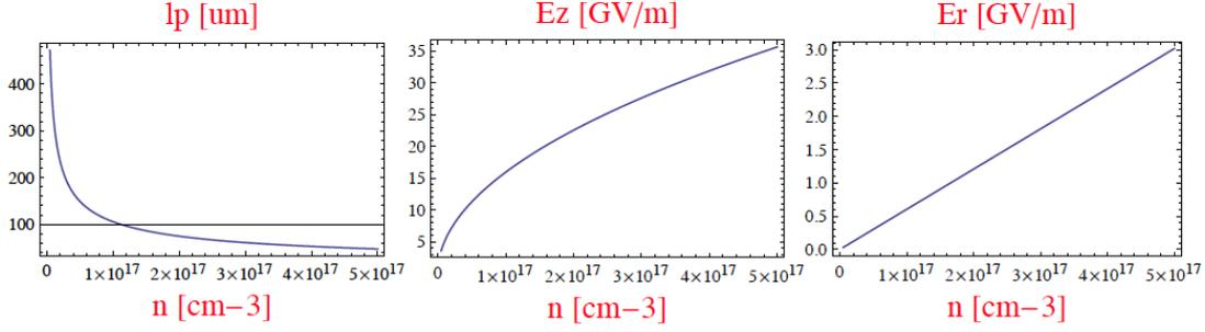
Fig. 10 - Plasma wavelength (left), longitudinal (center) and transverse (right) fields versus typical plasma densities experienced by a test particle located at  $x=1 \mu\text{m}$  and  $\zeta = \frac{\lambda_p}{4}$ .
