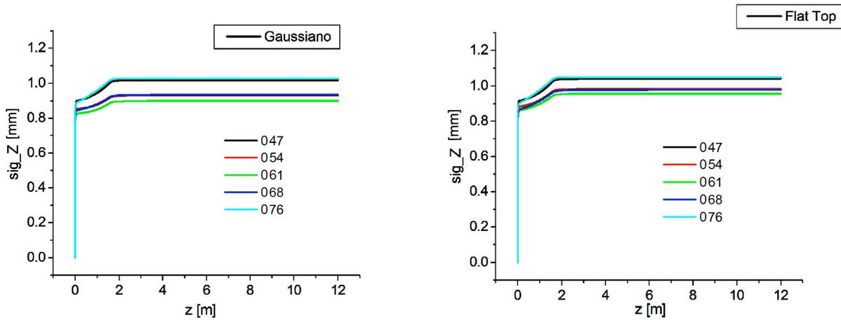
Figure 4 –  $\sigma_z$  of the beams along the SPARC linac, for Gaussian and flat-top distributions
