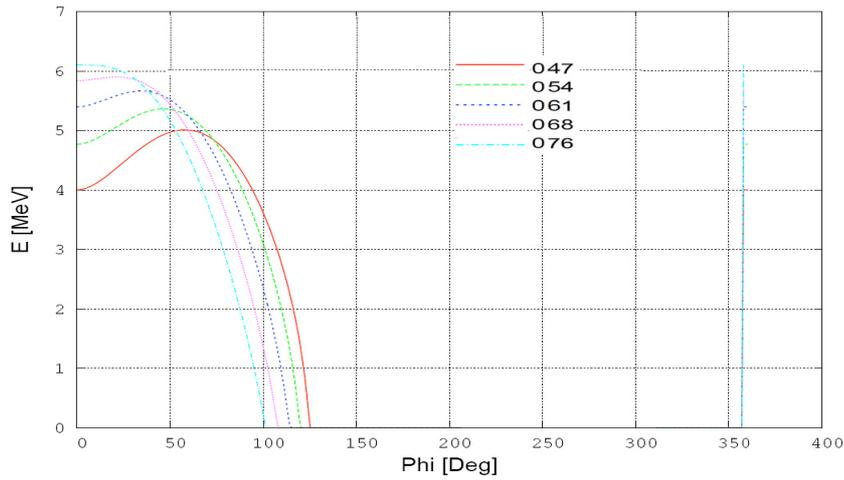
Figure 3 – Energy of the beam versus the injection phase for the Gaussian distribution
