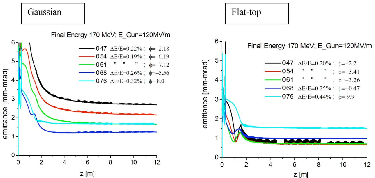
Figure 2 – Rms normalized emittance behaviour along the SPARC linac for a Gaussian bunch and for a flat-top bunch. Different colours show different HC lengths
