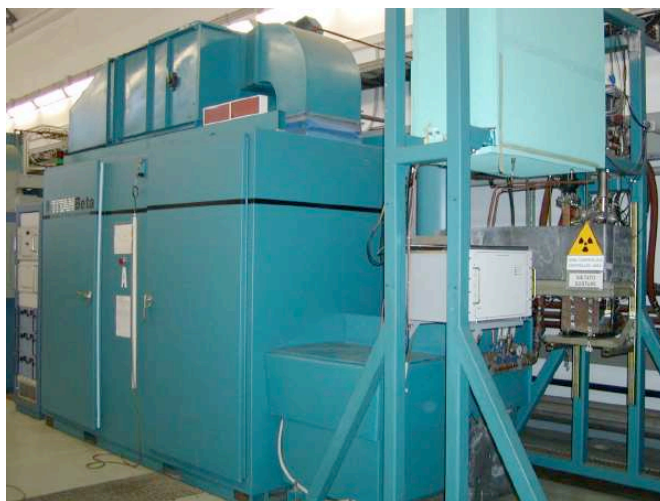
Figure 4.21. The power station of a S-band klystron, including high-voltage supply, pulse-forming network, and thyatron switch.
