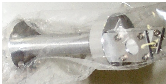
Figure 4.32: UCLA Ce:YAG detector and mirror, mounted on assembly.
