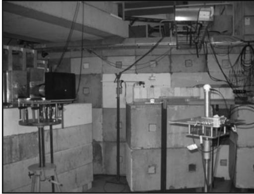
Figure 1. Picture of the irradiation facility at TSL. Thirty-eight mega-electronvolt protons were accelerated on a 5-mm water-cooled beryllium target. The neutron fields produced by the target bare and attenuated by a 10-cm polyethylene layer (see the black parallelepiped) irradiated the different spheres of the ERBSS (on the right side of the figure).
