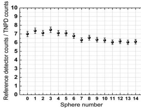
Figure 7. Ratio of the response of the reference <sup>6</sup>LiI(Eu) scintillator and the one of the TNPD at each sphere type. The value results to be  $6.53 \pm 0.70$ .
