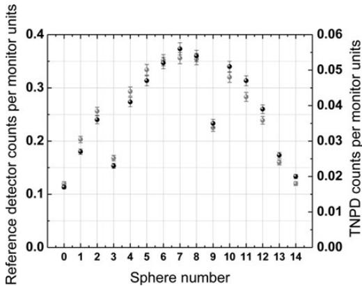
Figure 6. Counts per monitor unit obtained by irradiating with the attenuated neutron field the ERBSS equipped with the reference detector LiI(Eu) (grey points) and with the TNPD (black points).
