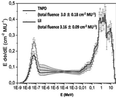
Figure 5. Total neutron field: spectral neutron fluence distribution per monitor units derived through the reference detector (grey line) and by the TNPD (black line). The total neutron fluence per monitor unit is also indicated.
