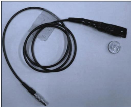
Figure 2. The thermal neutron pulse detector (TNPd).
