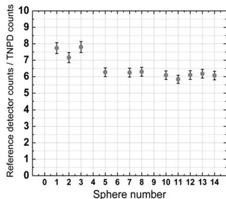
Figure 4. Ratio of the response of the reference  ${}^6\text{Li}(\text{Eu})$  scintillator and the one of the TNPd at each sphere type. The value results to be  $6.65 \pm 0.51$ .
