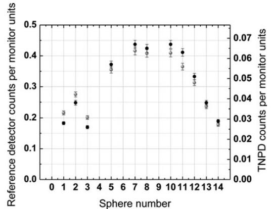
Figure 3. Counts per monitor unit obtained by irradiating with the total neutron field the ERBSS equipped with the reference detector LiI(Eu) (grey points) and with the TNPd (black points).
