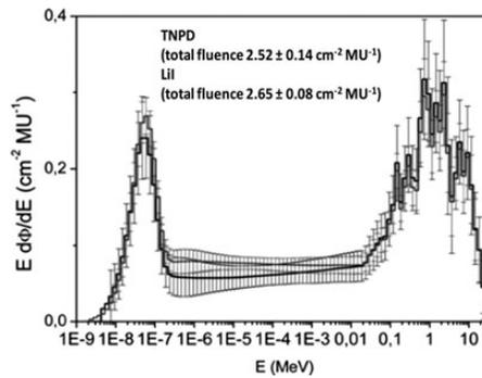
Figure 8. Moderated neutron field: spectral neutron fluence distribution per monitor units derived through the reference detector (grey line) and by the TNPD (black line). The total neutron fluence per monitor unit is also indicated.
