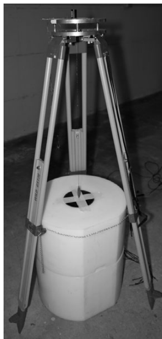
Figure 4. Irradiation set up for testing the CYSP. A dummy source is located on the top of the tripod holder. The boron-lined mouth of the CYSP's neutron collimator is visible.
