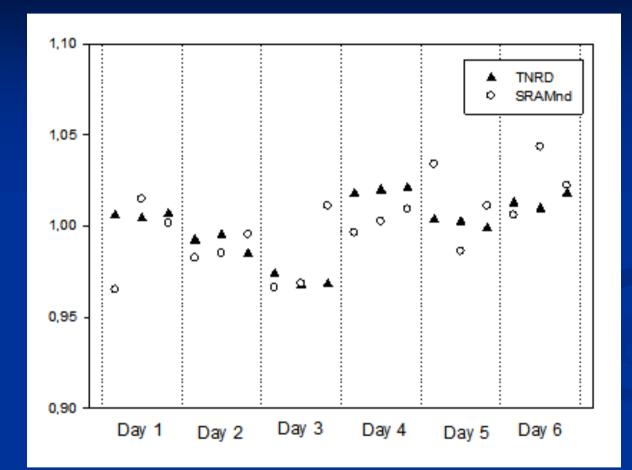
Multiple measurements with 1000 MU (Monitor Unit) performed with TNRD and SRAMnd; TNRD presents a standard deviation of 1.70%, better than the 2.21% of the SRAMnd.
