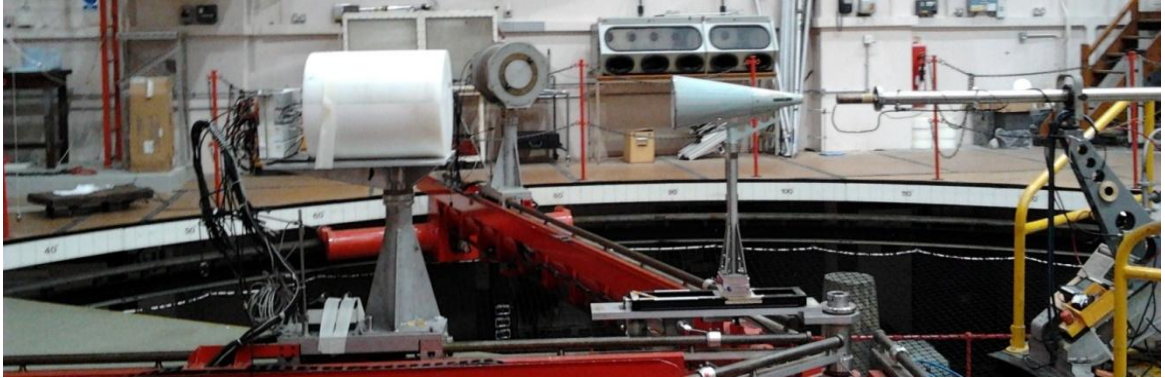
Figure 4.1: Experimental set-up. The distance from the neutron producing target to the end of the cylinder was equal to 150.5 cm.
