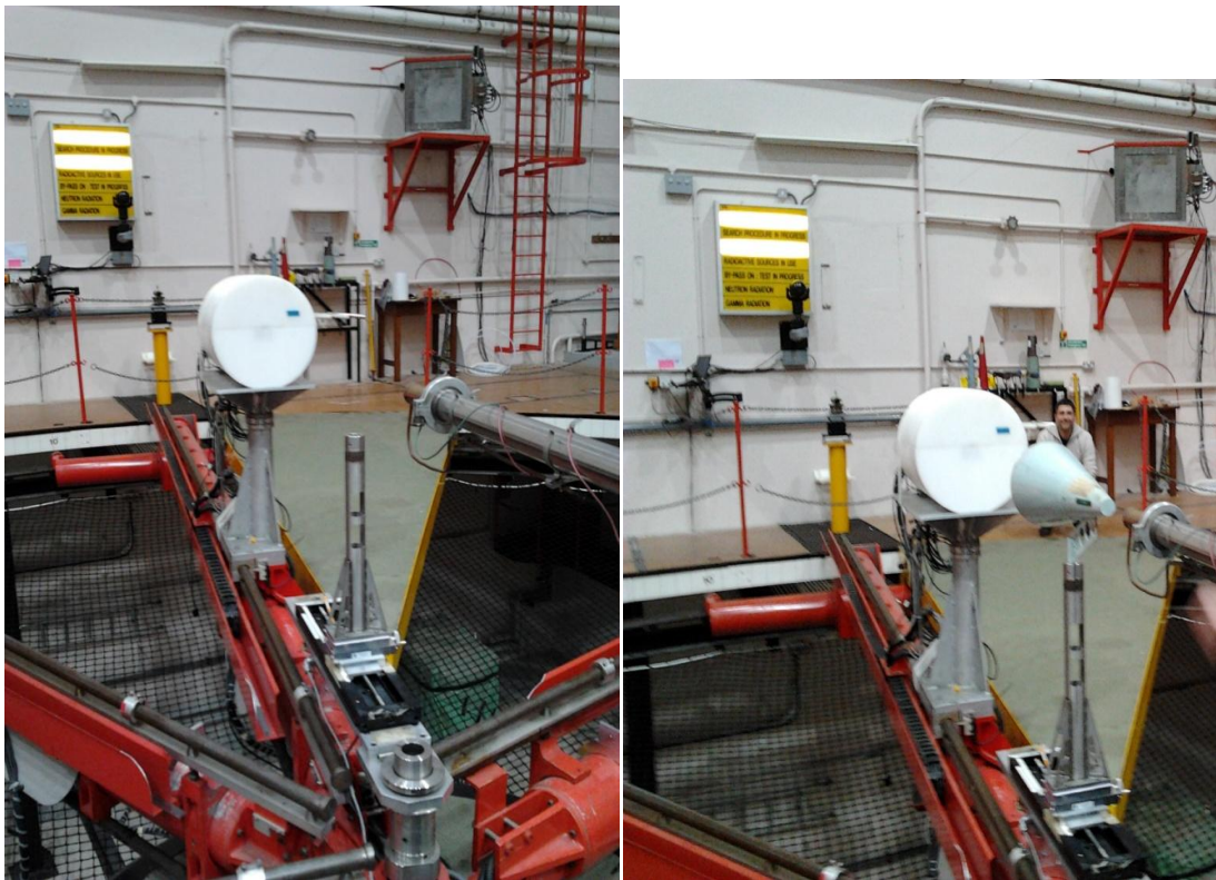
Figure 4.2: Experimental set-up for measurements of the total neutron field (left) and of the only scatter component by using a shadow cone (right).
