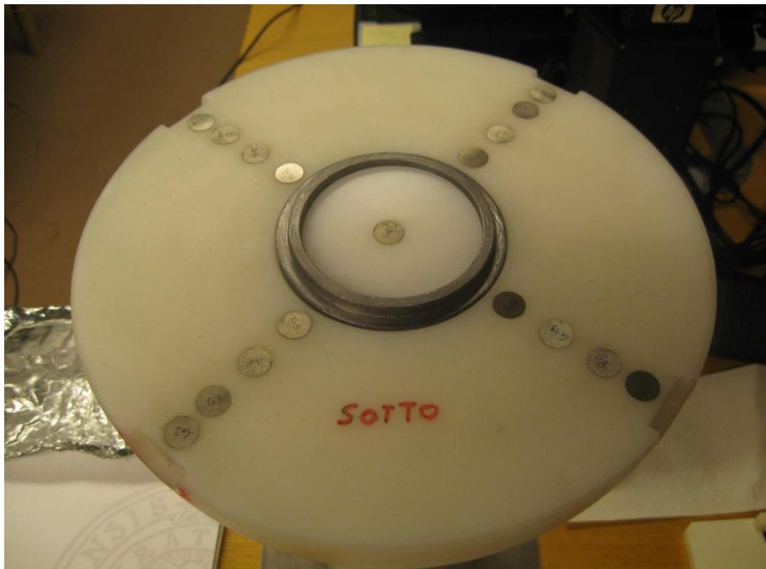
Figure 2.3: Schematic view and image of the internal part of the High-energy spectrometer, showing the arrangement of the activation foils detectors along three perpendicular axes, as well as the inner lead layer.
