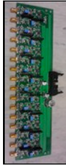
Figure 3. Multi-detector NESCOFI acquisition board. Up to 16 detectors can be controlled through SMA connectors. For every detector a charge preamplifier and a shaper amplifier allow adapting, gaussian-shaping and magnifying the charge pulses produced in the semiconductor based thermal neutron detectors. The amplified signals are sent to a multi-channel digitizer (NI USB 6366) controlled through a Labview program. The control software allows simultaneous spectrum calculation for all detectors.
