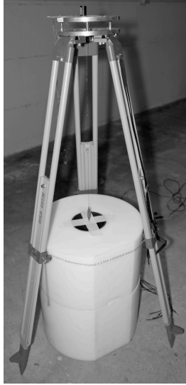
Fig. 15. Irradiation set-up of the CSYP at the INFN-LNF. The source is on top.
