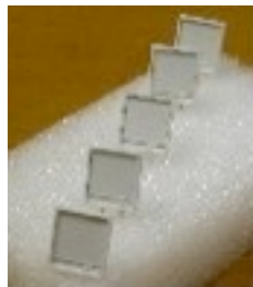
Figure 2. The ATNDs, after the in-house sensitization process. The white layer is the (n, charged particle) converter. The silicon diode detects the resulting charged particles.
