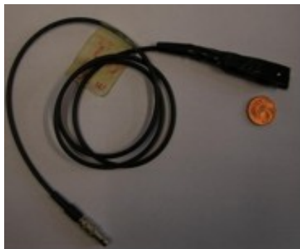
Figure 6.22. Left: The thermal neutron rate detector (TNRD). Right: Time-dependent output of the TNRD when exposed in an ex-core thermal neutron beam from the ENEA Casaccia TRIGA reactor at power 46 kW (thermal flux 6E+4 \text{ cm}^{-2}\text{s}^{-1} ).
