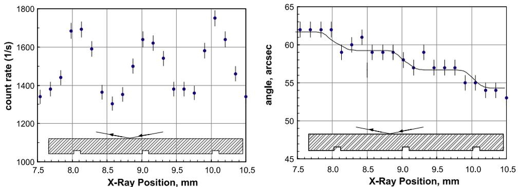
Fig. 16. Diffraction from the side without grooves: intensity (left) and angle (right) of the diffraction peak.
