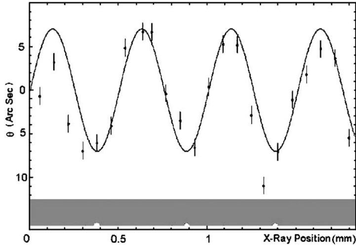
Fig. 19. X-ray test of one of the undulators.
