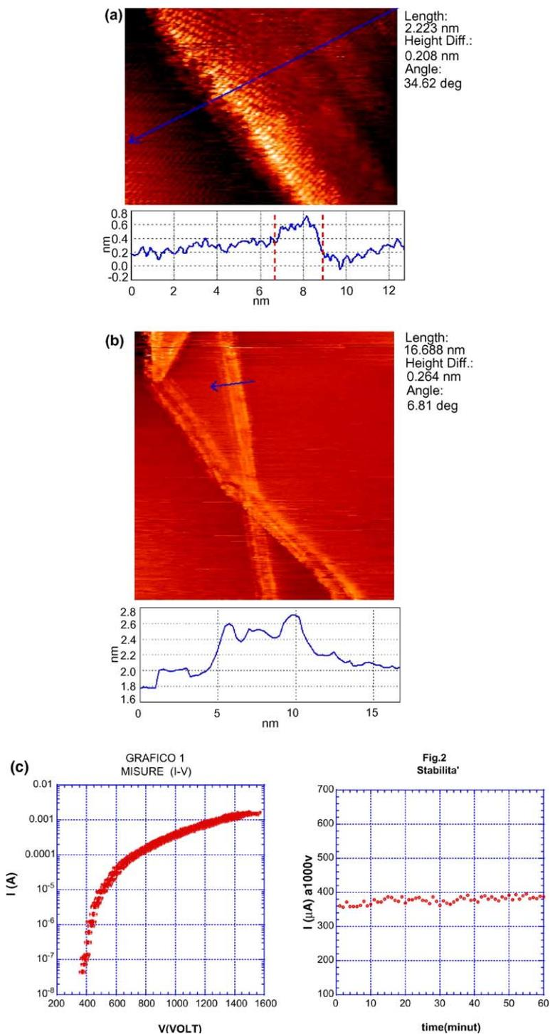
Fig. 10. (a) STM image of a SWNT on HOPG substrate. (b) STM image showing SWNT bundles crossing. (c) We analyzed the stability of the sample, collecting the emitted current for 1 h, for a constant value of the applied field 1000 V. In Graph 2 above (right) we report this measurement, yielding an average value ( $377 \pm 17$ )  $\mu\text{A}$ .
