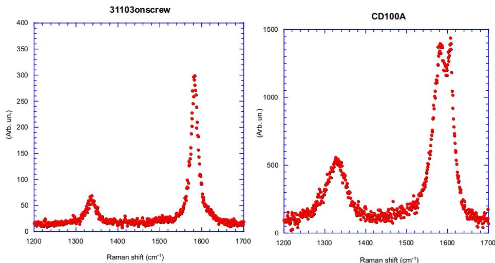
Fig. 6. D, G peaks in the Raman spectra of samples in Fig. 4.
