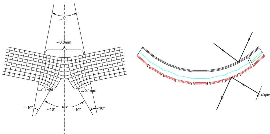
Fig. 18. Deformation of sample near groove reconstructed from X-ray measurements (left); deformation of the whole sample (right).
