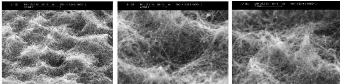
Fig. 2. SEM images of a nanotube carpet synthesized at INFN-LNF with a different arc-discharge setup, showing a very high ratio of nanotubes.
