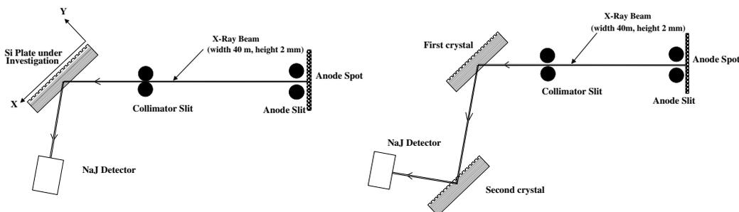
Fig. 14. Testing CU with X-rays at PNPI-St. Petersburg: one crystal (left) and two crystal (right) diffraction scheme.
