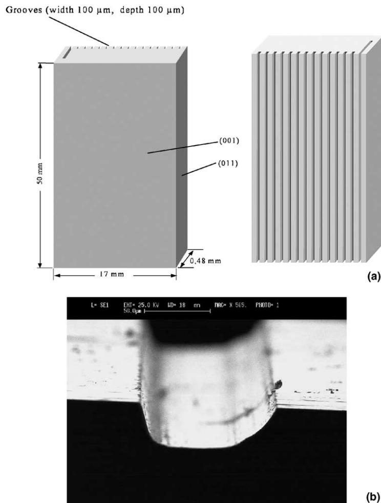
Fig. 11. (a) Schematic description of a sample prepared by U. Ferrara and IHEP-Protvino in Spring, 2002. (b) SEM image of a microgroove on the crystal surface.
