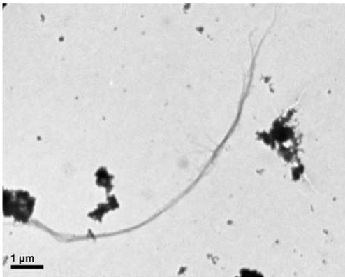
Fig. 3. TEM images of a carbon nanotube bundle obtained by arc discharge at INFN-LNF, shown on scales of 1  $\mu\text{m}$ .
