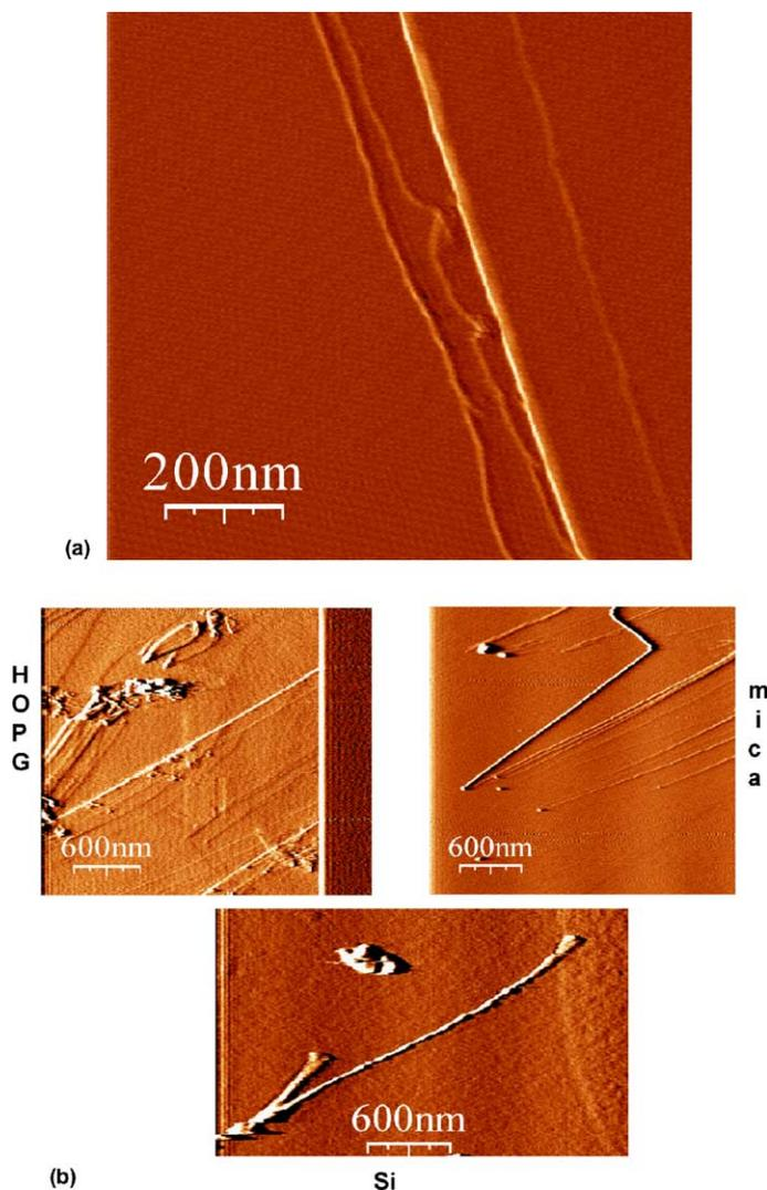
Fig. 7. (a) AFM image of CNT synthesized by arc discharge showing bundles of MWNT. (b) AFM images of CNT on (a) HOPG, (b) mica and (c) silicon surface.
