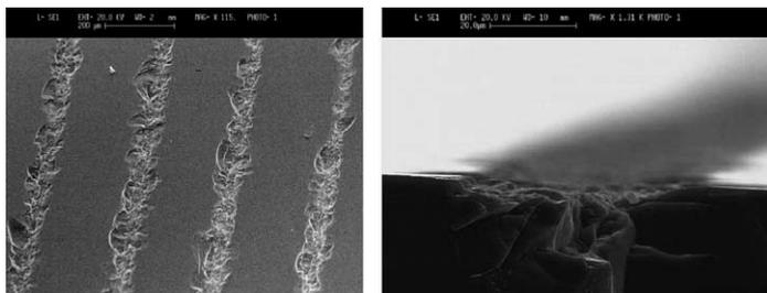
Fig. 12. SEM images of a Si CU showing 50  $\mu\text{m}$  grooves spaced by 200  $\mu\text{m}$  on the undulator surface obtained at IHEP-Protvino; the side view on the left shows how micromachining produces periodical deformations that propagate in the bulk of the crystal.
