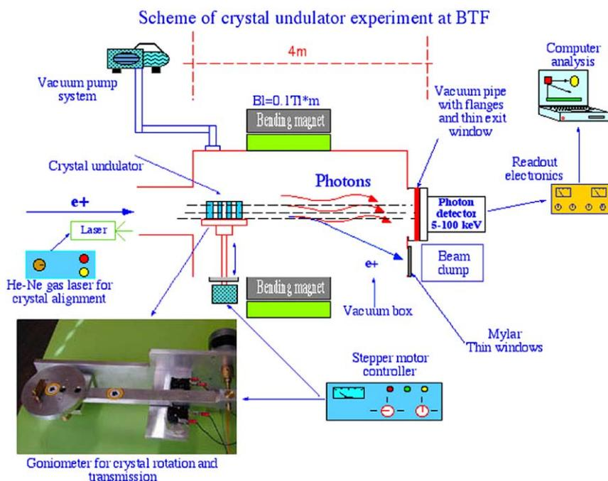
Fig. 21. The layout of the LNF experiment on photon emission in crystalline undulators.
