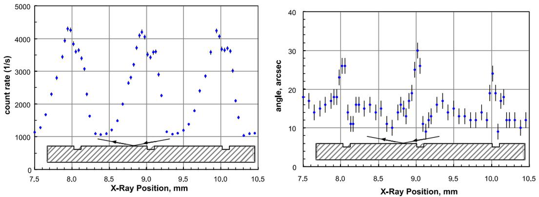
Fig. 15. Diffraction from the side with grooves: intensity (left) and angle (right) of the diffraction peak.
