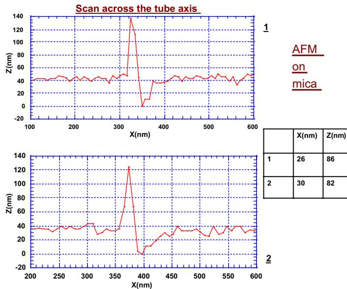
Fig. 9. AFM image shows a lateral elongation of the nanotube (due to strong interaction between the tip and the tube surface).
