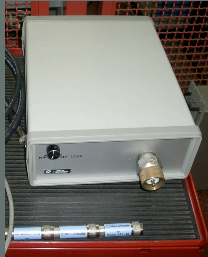
The 24kV FID used for lab HV tests
