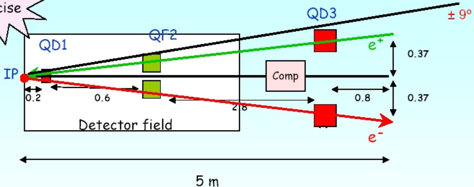
With  $\pm 10\sigma_x$  clearance,  $\pm 9^\circ$  cone,  $\pm 30$  mrad angle:
