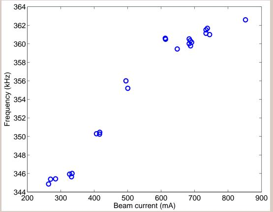
A fast increase in tune between 350 and 600 kHz, then saturation
