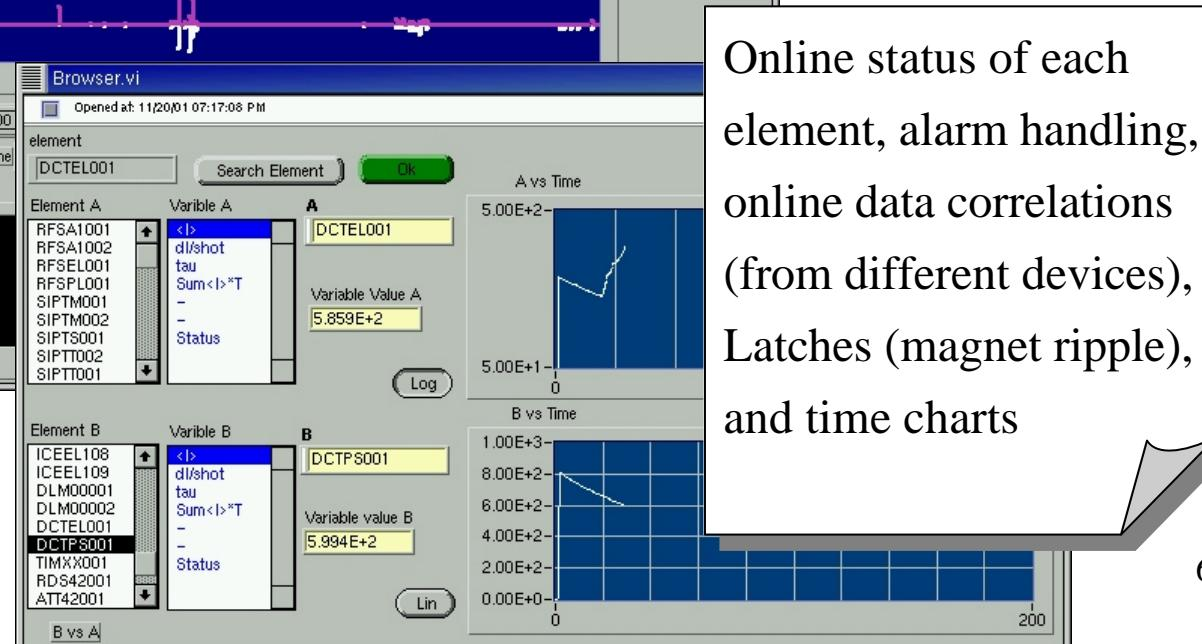
Online status of each element, alarm handling, online data correlations (from different devices), Latches (magnet ripple), and time charts
