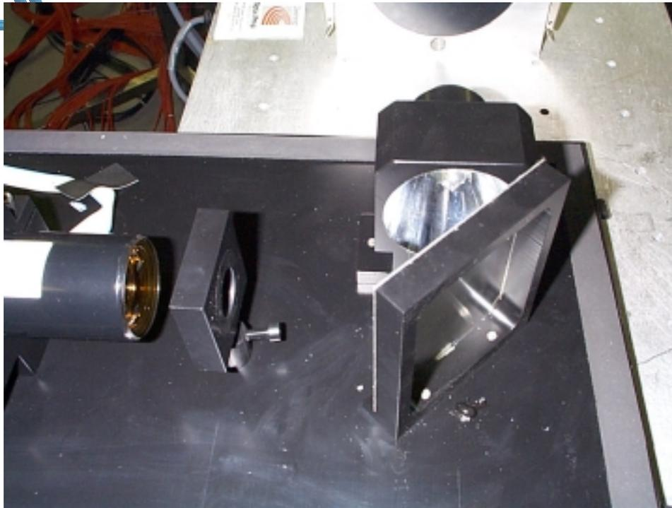
The Cerenkov light is extracted from the plexiglass radiator by appropriate shaping of the end part without optical connection to the PMT. Calibrated attenuating filters allow the measurement of the beam intensity over several order of magnitudes. Inter-calibration with the calorimeter
