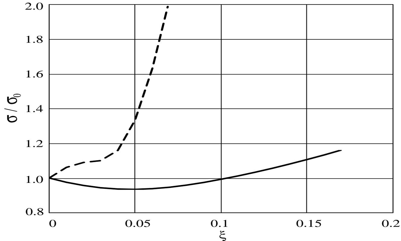
**Vertical beam size vs. the beam-beam parameter.
