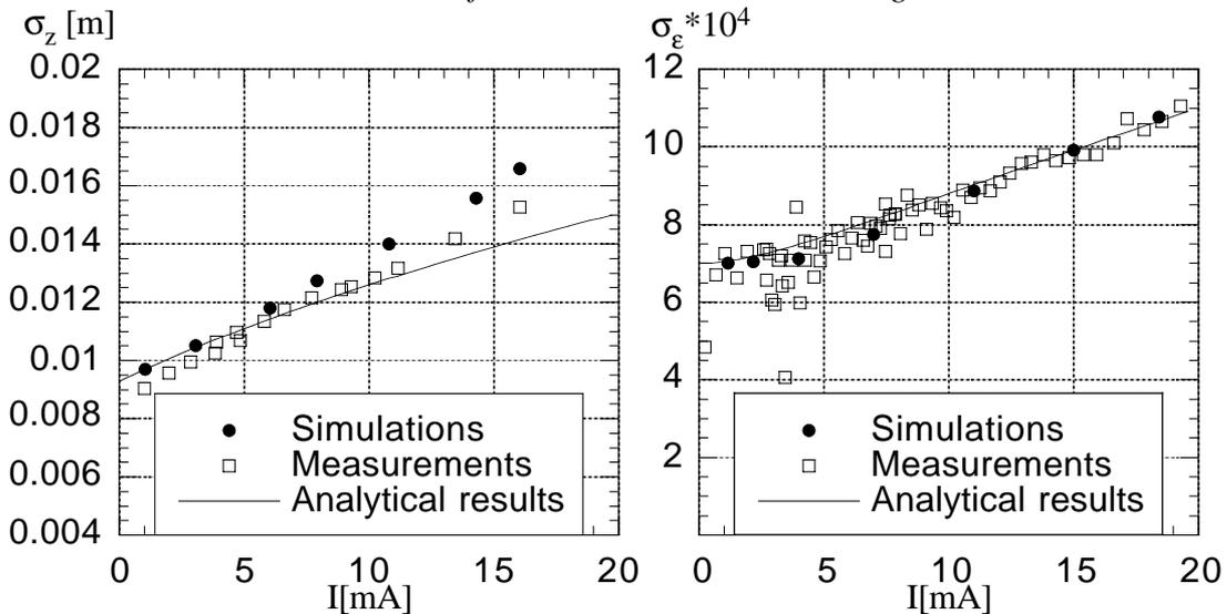
Figure 2: Bunch length at  $v_s = 3.77 \cdot 10^{-3}$  and energy spread at  $v_s = 7.71 \cdot 10^{-3}$  vs current for ALS machine (by courtesy of J. Byrd).
