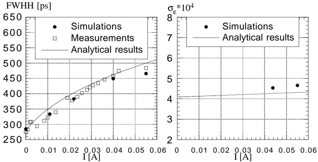
Figure 1: Full width half high and energy spread vs current for DAΦNE Accumulator Ring.
