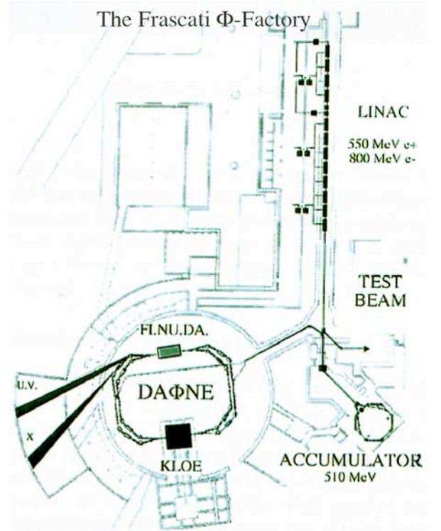
Figure 1: Layout of DAΦNE and its injector
