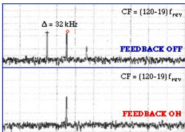
Figure 5: Beam spectrum without and with feedback in the positron ring, 30 bunches, 70 mA
