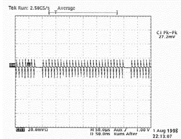
Figure 6: Typical positron fill (the gap of two missing bunches separates two successive revolutions).
