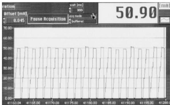
Figure 3: A typical injection/extraction cycle as seen on the DCCT monitor
