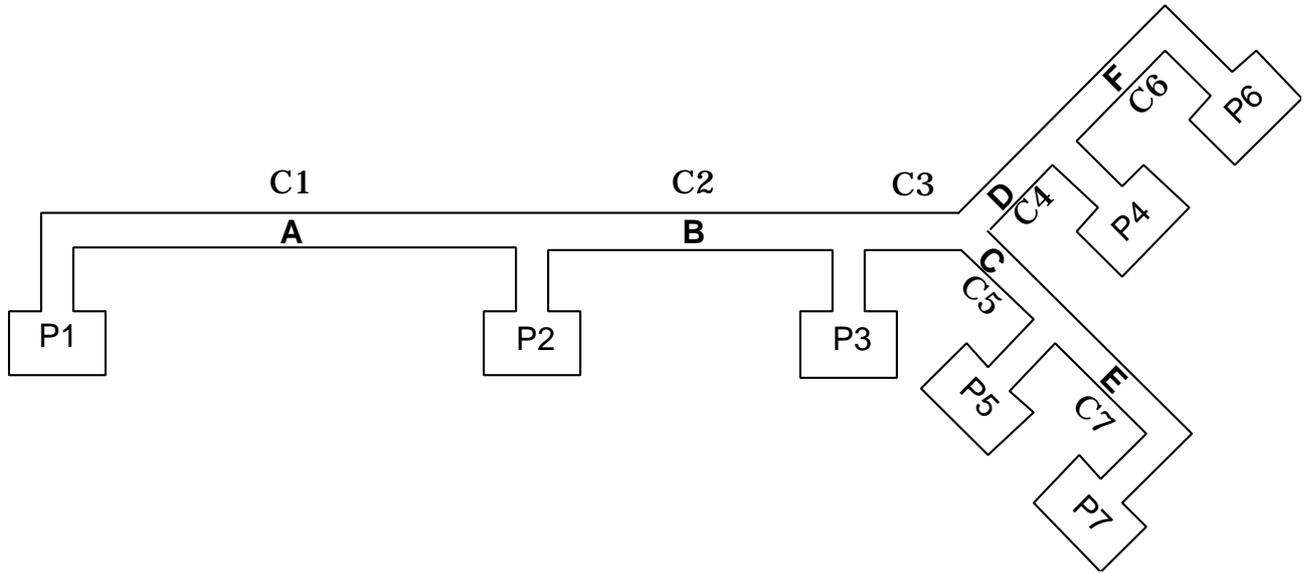
*Fig. 2 - Schematic drawing of the transfer lines vacuum system.*
