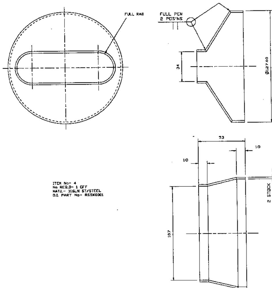
Fig. 3a - Shallow cavity initial part.
