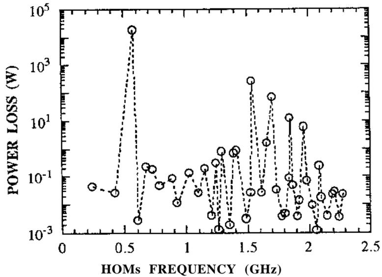
Fig. 1 - Power losses versus mode frequency.
