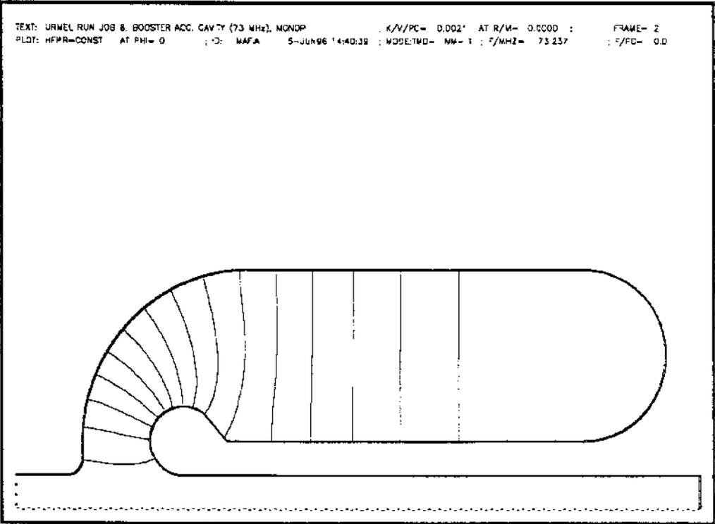
Fig. 6 - Electric field flux lines distribution of the fundamental mode.
