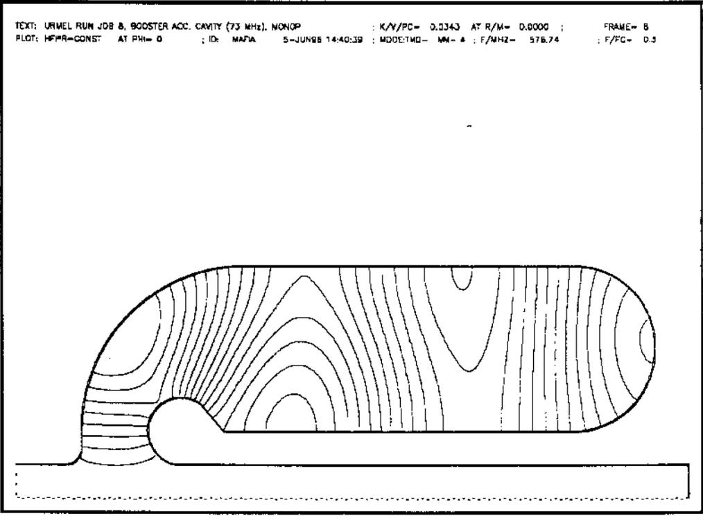
Fig. 7 - Electric field flux lines distribution of the dangerous parasitic HOM mode.
