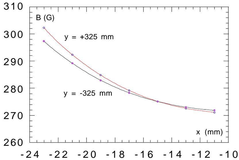
*Figure 8 - Horizontal dependence of the vertical field at  $\pm 25$  mm outside the magnet yoke boundary*
