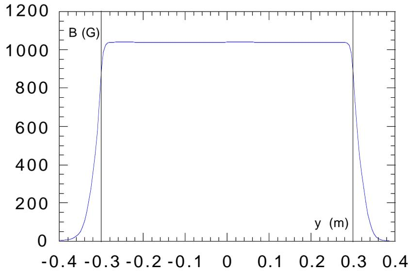
*Figure 4 - Magnetic field at the centre of the magnet gap.
