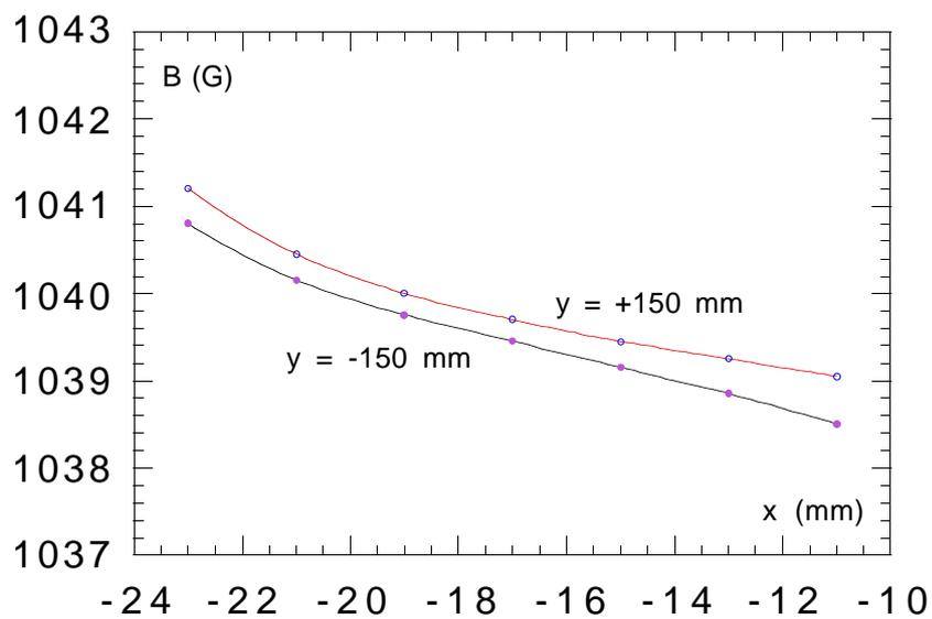
*Figure 6 - Horizontal dependence of the vertical field at  $\pm 150$  mm from magnet centre*
