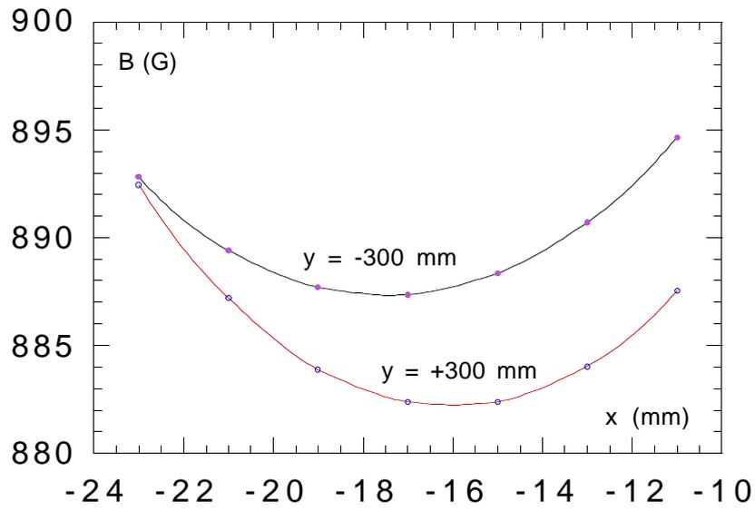
*Figure 7 - Horizontal dependence of the vertical field at  $\pm 300$  mm from magnet centre (yoke boundary)*
