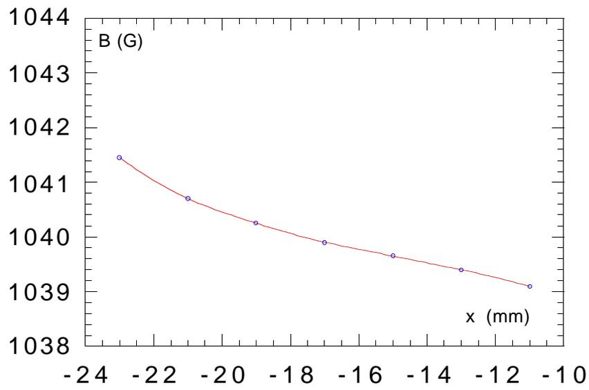
*Figure 5 - Horizontal dependence of the vertical field at magnet centre*
