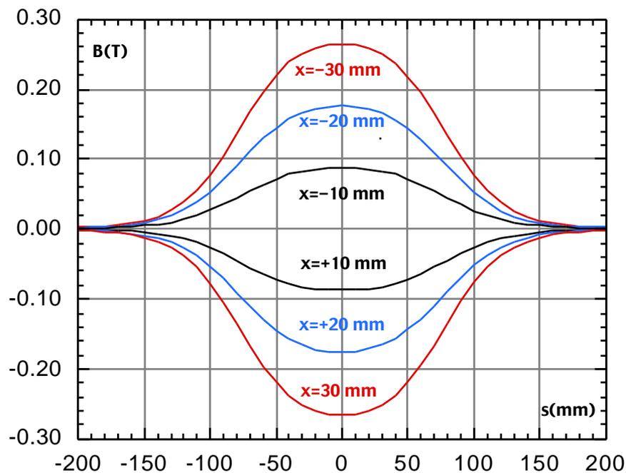
Figure 4 - Longitudinal field behaviour along straight lines parallel to the quadrupole axis. Quadrupole Q1 sn#2
