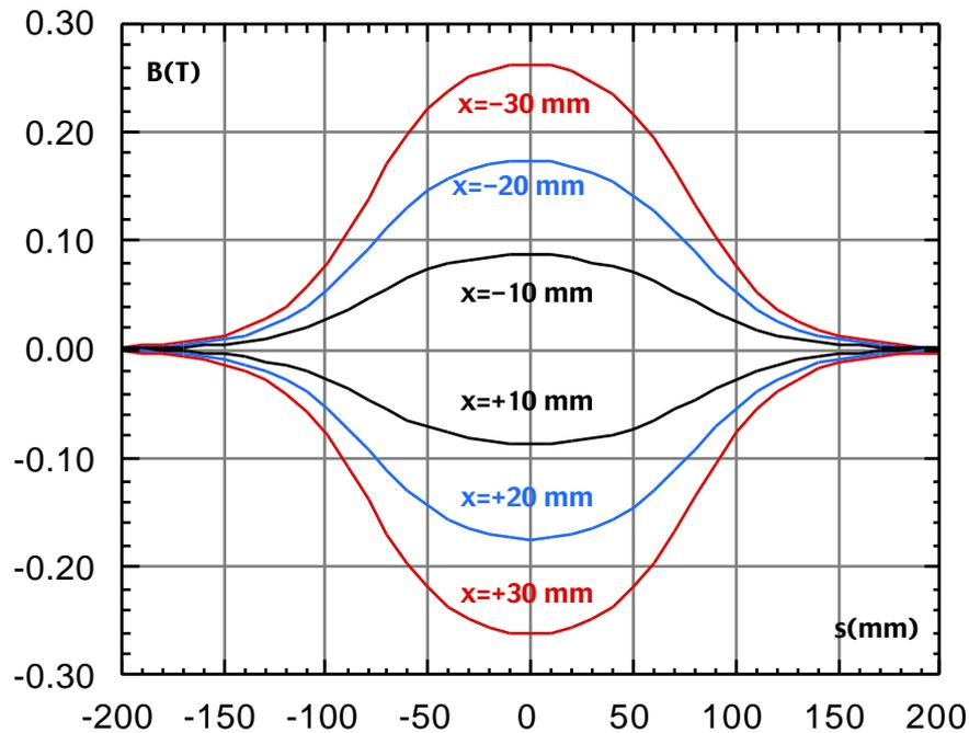
Figure 3 - Longitudinal field behaviour along straight lines parallel to the quadrupole axis. Quadrupole Q1 sn#1
