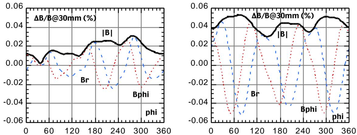
Figure 1 - Relative deviation from ideal quadrupole field @ 30 mm from magnet axis:
