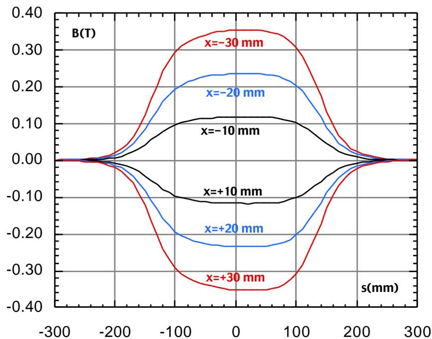
Figure 8 - Longitudinal field behaviour along straight lines parallel to the quadrupole axis. Quadrupole Q2 sn#4
