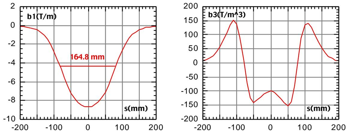
Figure 5 - Fitted gradient and third order term of the transverse expansion of the field measured on the horizontal symmetry plane for Q1 sn#1
