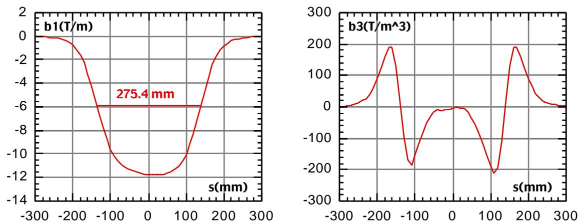
Figure 10 - Fitted gradient and third order term of the transverse expansion of the field measured on the horizontal symmetry plane for Q2 sn#4
