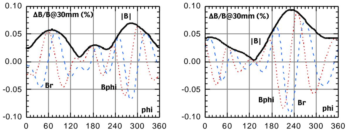
Figure 2 - Relative deviation from ideal quadrupole field @ 30 mm from magnet axis:
