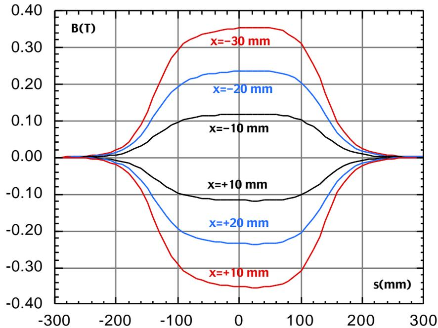
Figure 7 - Longitudinal field behaviour along straight lines parallel to the quadrupole axis. Quadrupole Q2 sn#3
