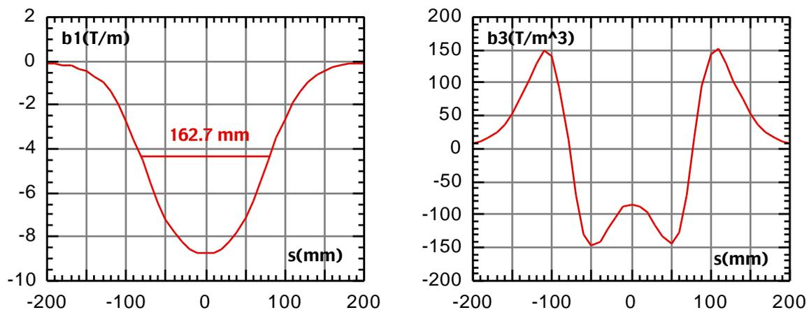
Figure 6 - Fitted gradient and third order term of the transverse expansion of the field measured on the horizontal symmetry plane for Q1 sn#2
