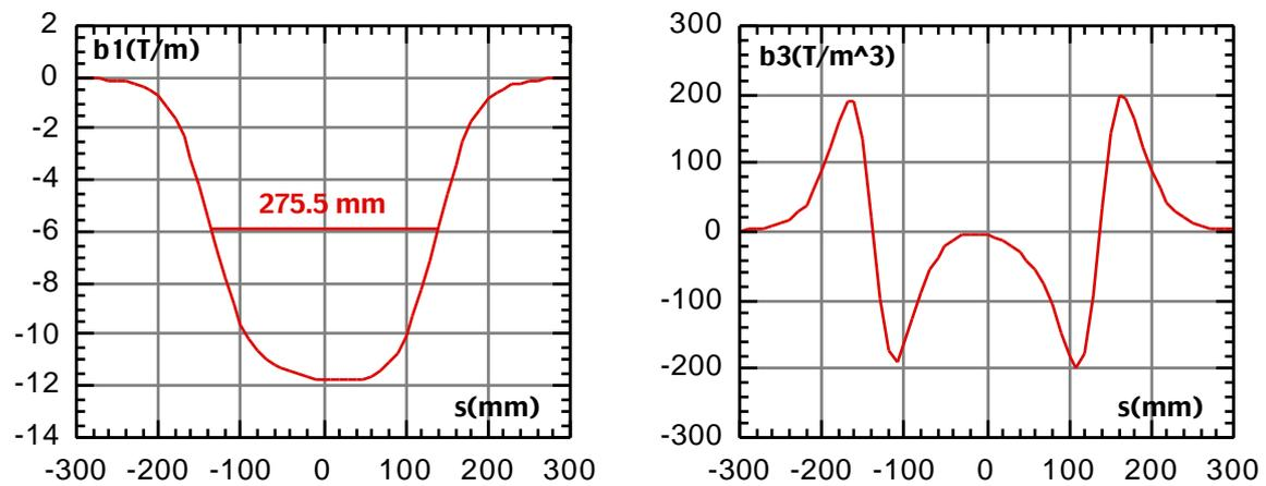
Figure 9 - Fitted gradient and third order term of the transverse expansion of the field measured on the horizontal symmetry plane for Q2 sn#3
