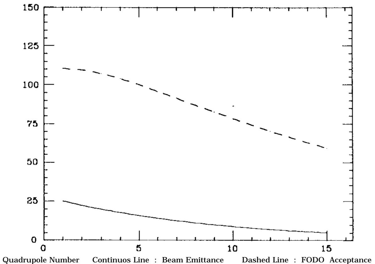
**Fig. 4** - Beam emittance and FODO acceptance of the DAΦNE positron Linac.
