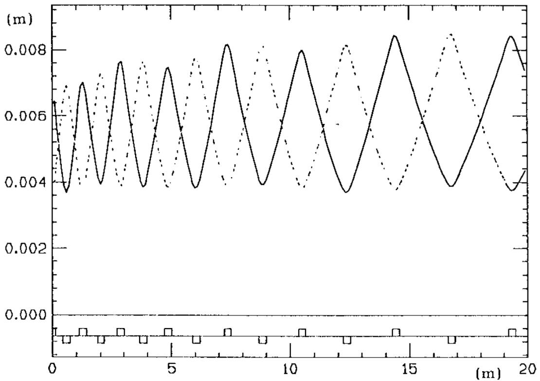
**Fig. 3** - Envelopes  $R_X$  and  $R_Z$  as calculated by the program LEDA using the FODO parameters calculated by the program FODO -  $R_X$  : continuous line;  $R_Z$  : dashed line.
