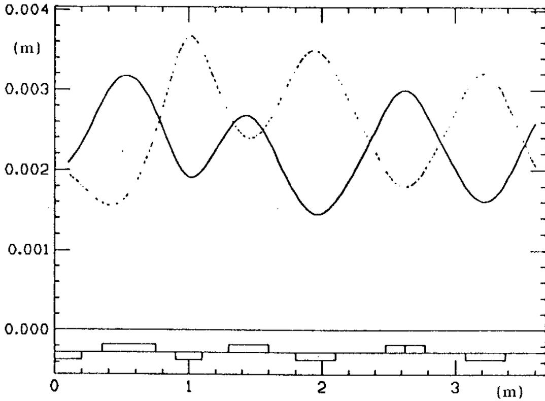
**Fig. 8** - Matching transition for DAΦNE FODO focusing in the case of electrons  $\varepsilon = 5\pi 10^{-6}$  m rad (@ 100 MeV) -  $R_X$  : continuous line;  $R_Z$  : dashed line
