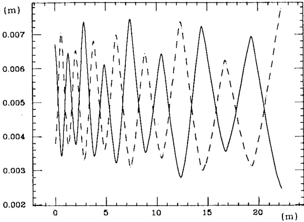
FODO for DAFNE positron LINAC  $R_X$  : continuous  $R_Z$  : dshed line
