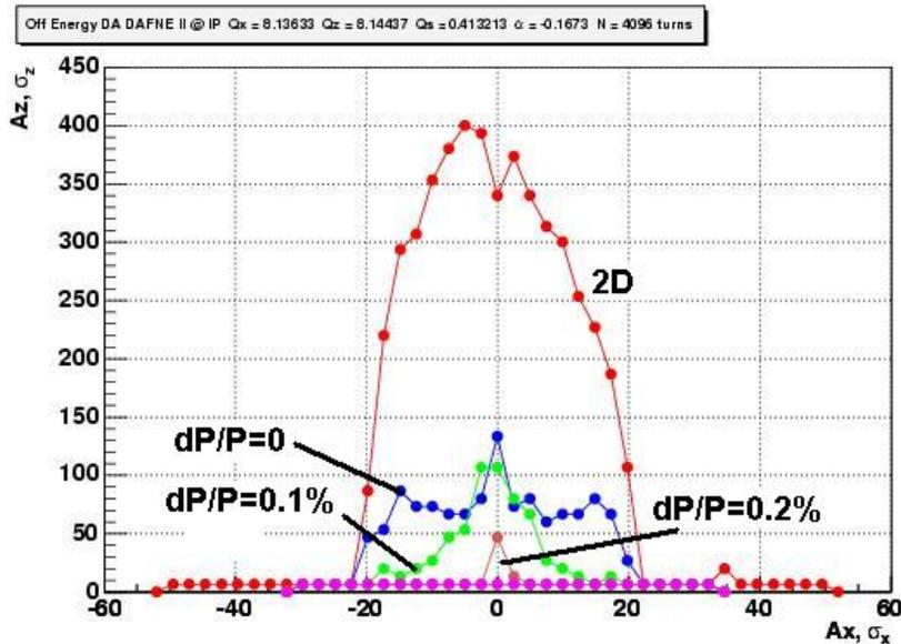
Figure 5 - A 3D dynamic aperture for  $Q_x = 8.136$  and  $Q_z = 8.144$ .
