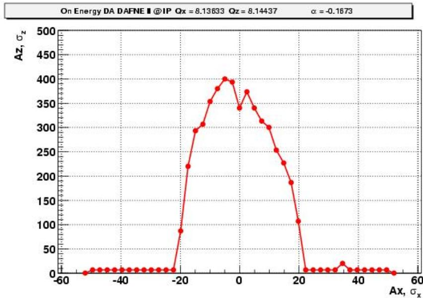
Figure 1 – The on-energy dynamic aperture. Note that the large horizontal DA shrinks when an arbitrary small vertical amplitude appears.
