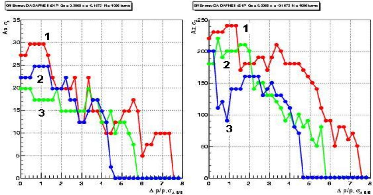
Figure 8 - Horizontal and vertical dynamic aperture as a function of the synchrotron oscillation amplitude for 3 tune points.
