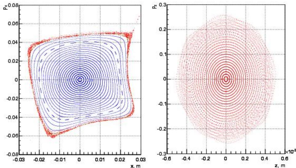
Figure 2 - The on-energy phase space portrait (horizontal and vertical).
