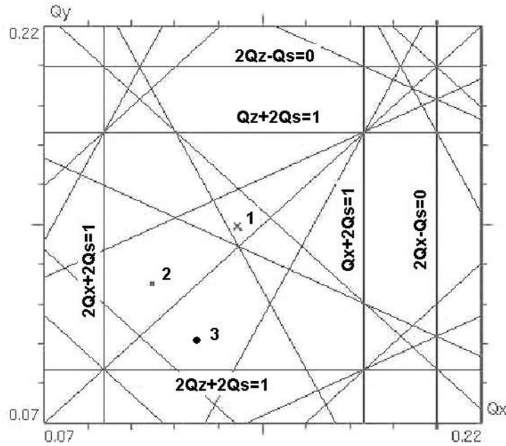
Figure 3 - Tune diagram (only the synchro-betatron satellite lines are shown). Three tune points are: 1 ( $Q_x = 8.136, Q_z = 8.144$ ), 2 ( $Q_x = 8.107, Q_z = 8.121$ ) and 3 ( $Q_x = 8.120, Q_z = 8.102$ ).
