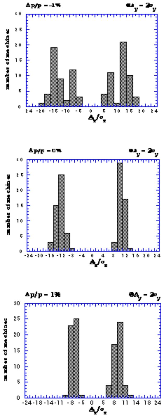
Fig. 5 - Day-one Lattice: effect of random multipole errors in all magnets including the low- $\beta$  quadrupoles, on a sample of 50 machines, for three energy deviations.
