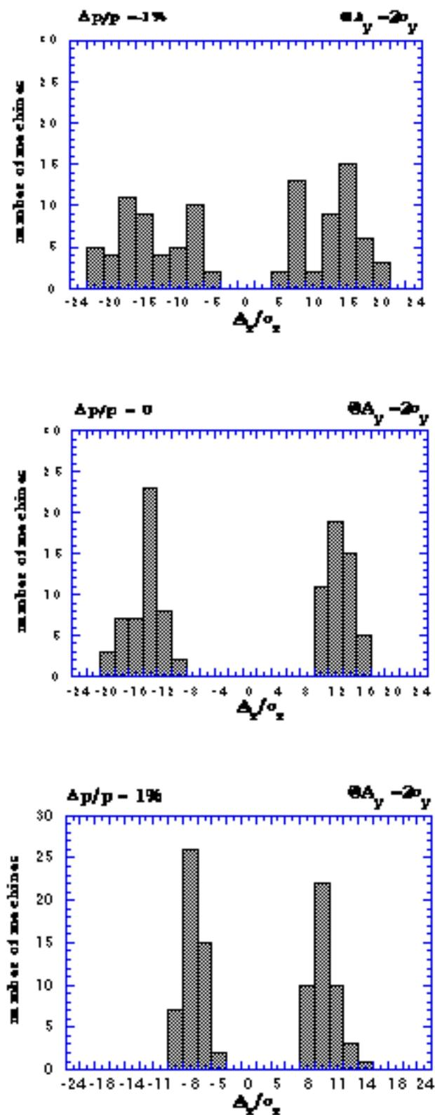
Fig. 4 - DAY-ONE Lattice: effect of random multipole errors in all magnets except for low- $\beta$  quadrupoles, on a sample of 50 machines, for three energy deviations.
