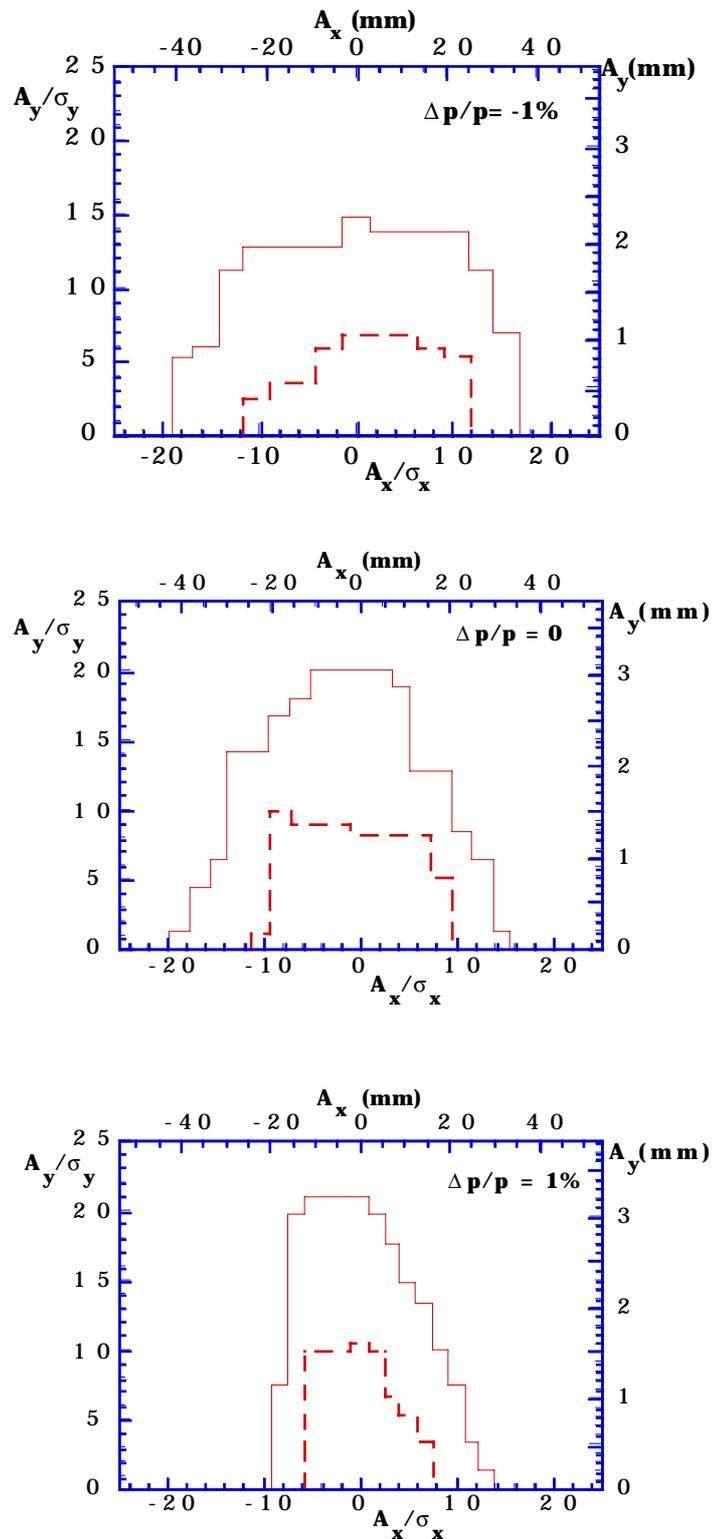
**Fig. 1** - Day-one Lattice: effect of systematic multipoles. Ideal dynamic aperture (solid line) compared to the one with all the systematic errors (dashed line) for three energy deviations.
