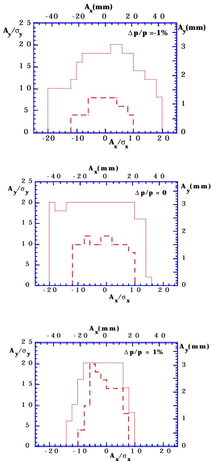
**Fig. 2** - D15 Lattice: effect of systematic multipoles. Ideal dynamic aperture (solid line) compared to the one with all the systematic errors (dashed line) for three energy deviations.
