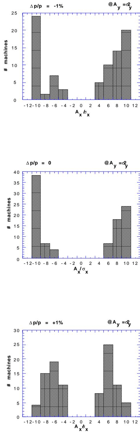
**Fig. 6** - D15 Lattice: effect of random multipole errors in all magnets including the low- $\beta$  quadrupoles, on a sample of 50 machines, for three energy deviations.
