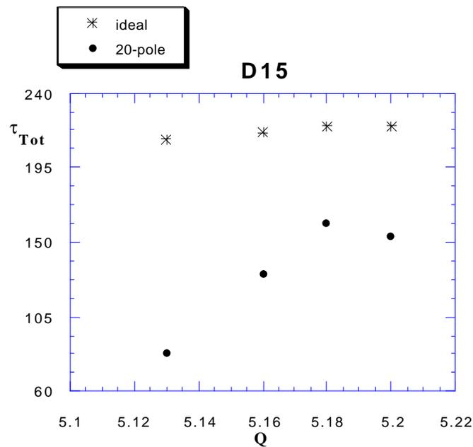
**Fig. 3** - D15 Lattice: dynamic aperture behaviour vs. horizontal tune for the ideal case (stars) and with 20-pole errors in low- $\beta$  quads only (dots).
