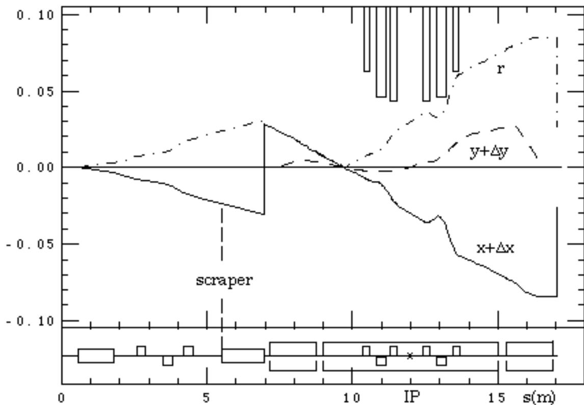
**Fig. 3** -  $x+\Delta x$ ,  $y+\Delta y$  and  $r$  from the bending upstream KLOE to the end of the KLOE IR, for  $\epsilon=-.0065$  and  $\theta=12.5\text{mrad}$ .
