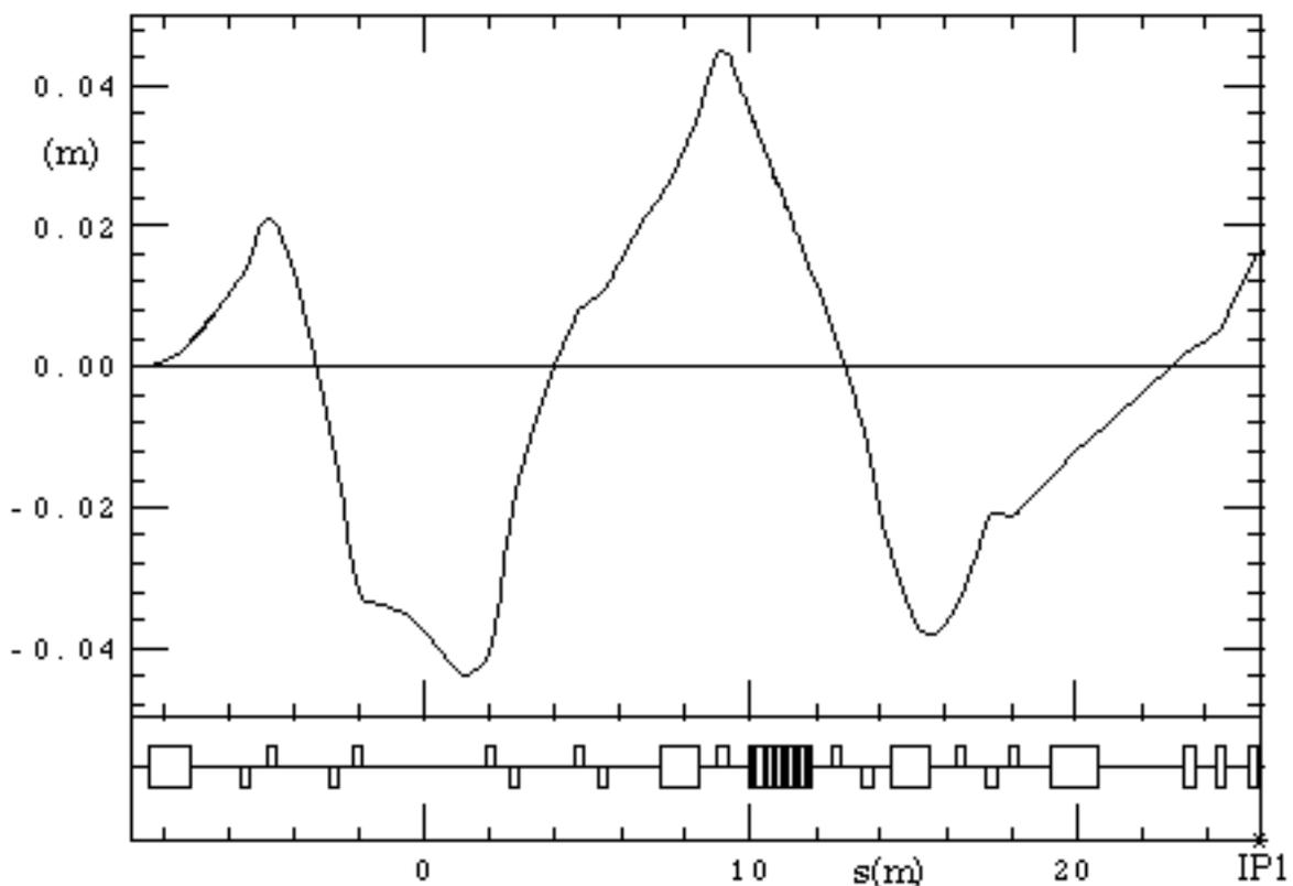
**Fig. A1** -  $x(\epsilon=.0065)$  from the bending upstream the LONG straight section to the KLOE IP.
