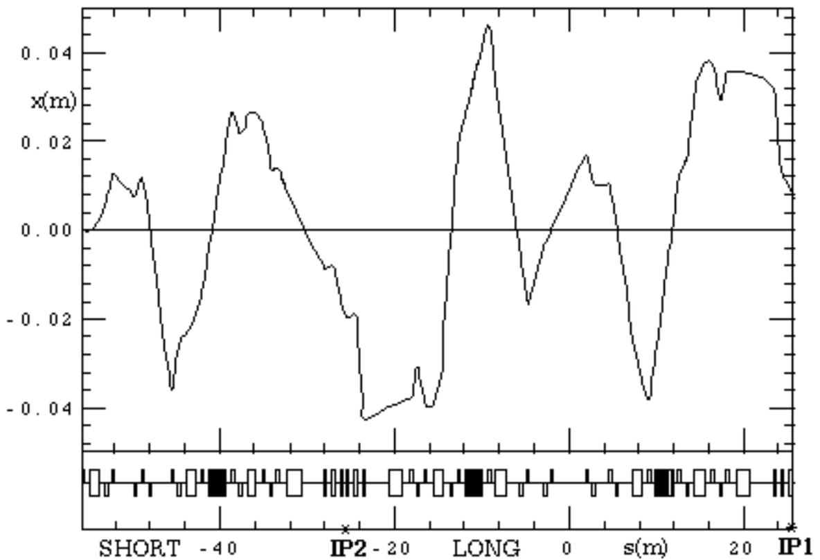
**Fig. A3** -  $x(\epsilon=.0065)$  from the bending upstream the SHORT straight section to the KLOE IP.
