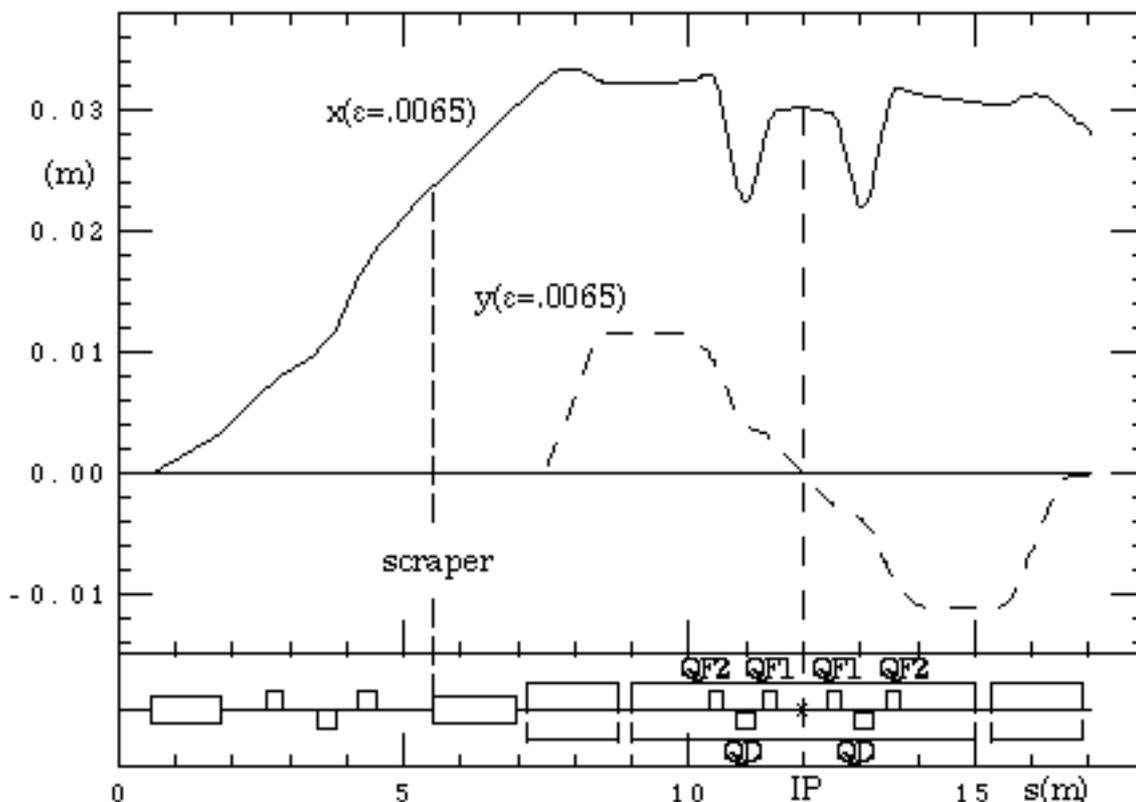
**Fig. 1** -  $x$  and  $y$  from the bending upstream KLOE to the end of the KLOE IR for  $\varepsilon = .0065$ .
