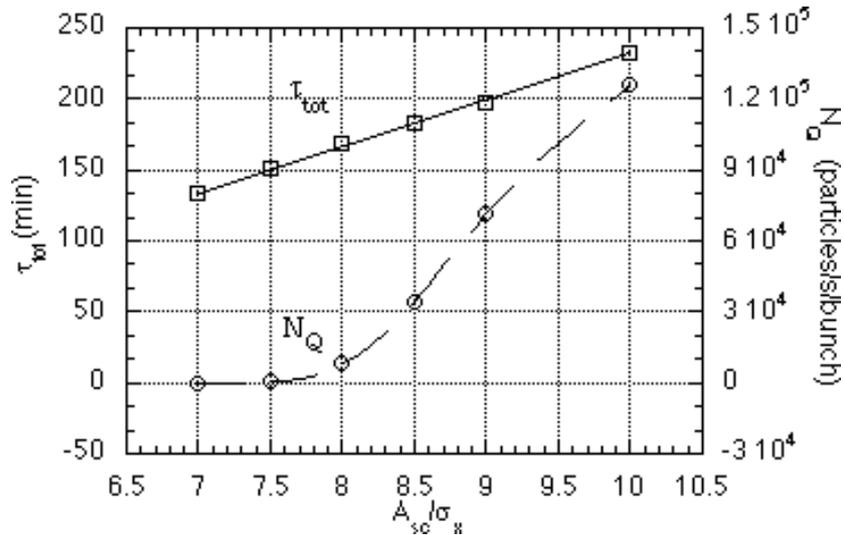
**Fig. 5** -  $\tau_{tot}$  and  $N_Q$  versus the scraper half aperture (in units of  $\sigma_x$  at the scraper).
