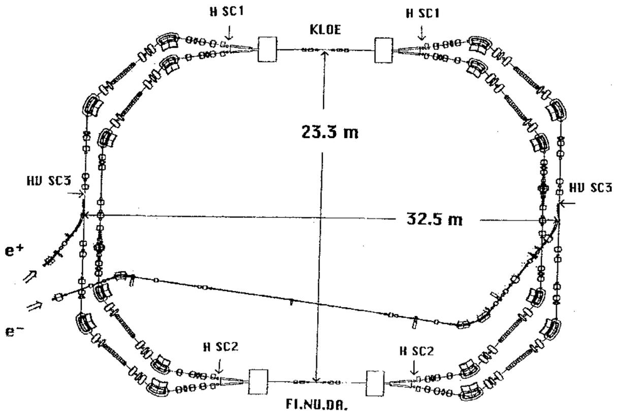
Fig. 4 - Location of the scrapers in the two rings.
