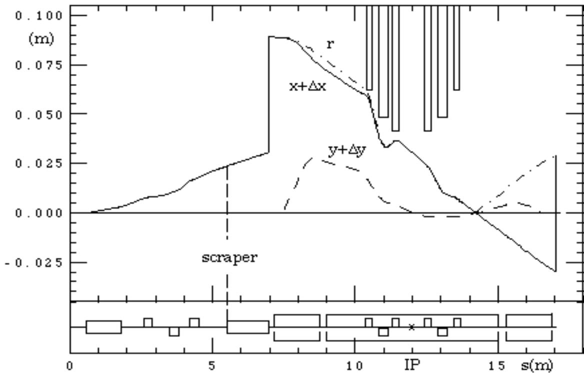
**Fig. 2** -  $x+\Delta x$ ,  $y+\Delta y$  and  $r$  from the bending upstream KLOE to the end of the KLOE IR, for  $\epsilon=.0065$  and  $\theta=12.5\text{mrad}$ .
