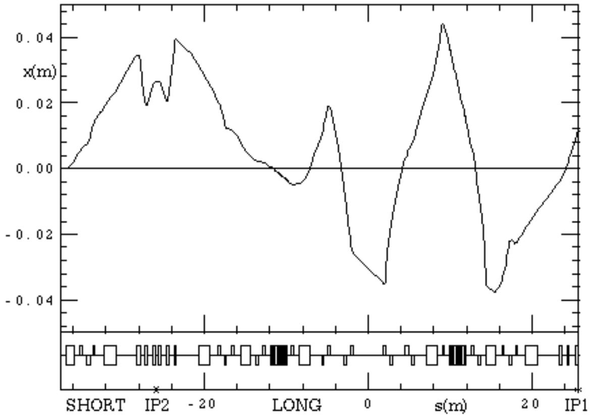
**Fig. A2** -  $x(\epsilon=.0065)$  from the bending upstream the FINUDA IR to the KLOE IP.
