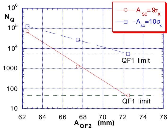
**Fig. 6** -  $N_Q$  as a function of the aperture of QF2 for two values of  $A_{sc}$  and  $\theta=12.5$ mrad.
