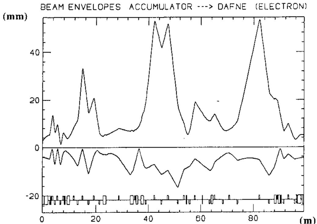
*Fig. 5-b: The horizontal and vertical beam-envelope as a function of distance for the **electron** 'OUT' beam. The beam-emittance for each plane is  $3 \times 10^{-7} \text{ m.rad.}$ .*
