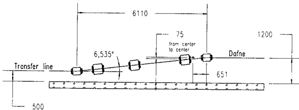
Fig. 1-b: The side views of vertical bends in the parts of lines.
