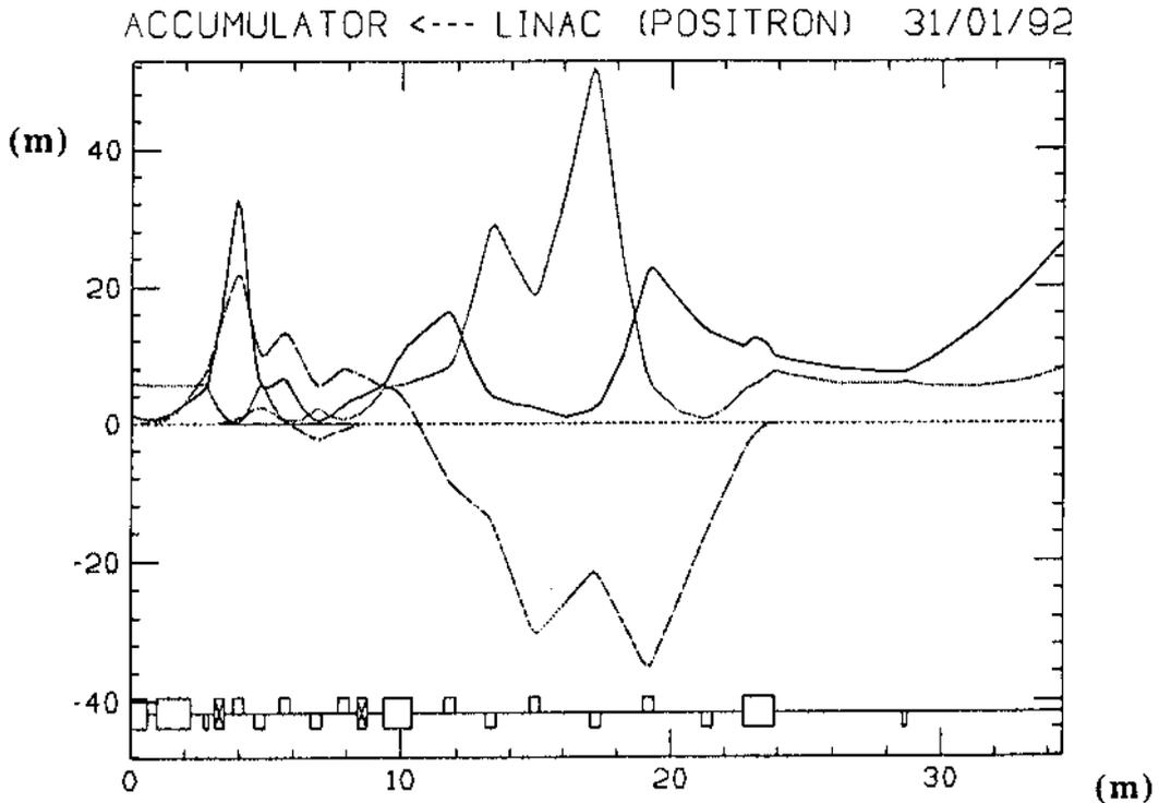
**Fig. 2-a:** The optical functions of **positron** 'IN' beam to the accumulator (the left side).
