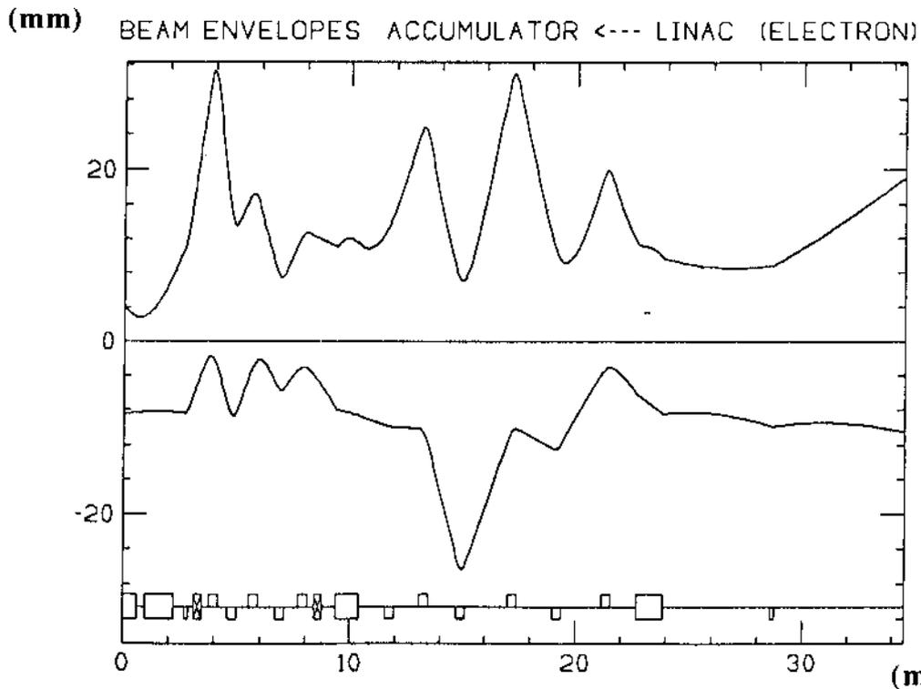
Fig. 3-b: The horizontal and vertical beam-envelope as a function of distance for the **electron** 'IN' beam. The beam-emittance for each plane is  $3 \times 10^{-7}$  m.rad..
