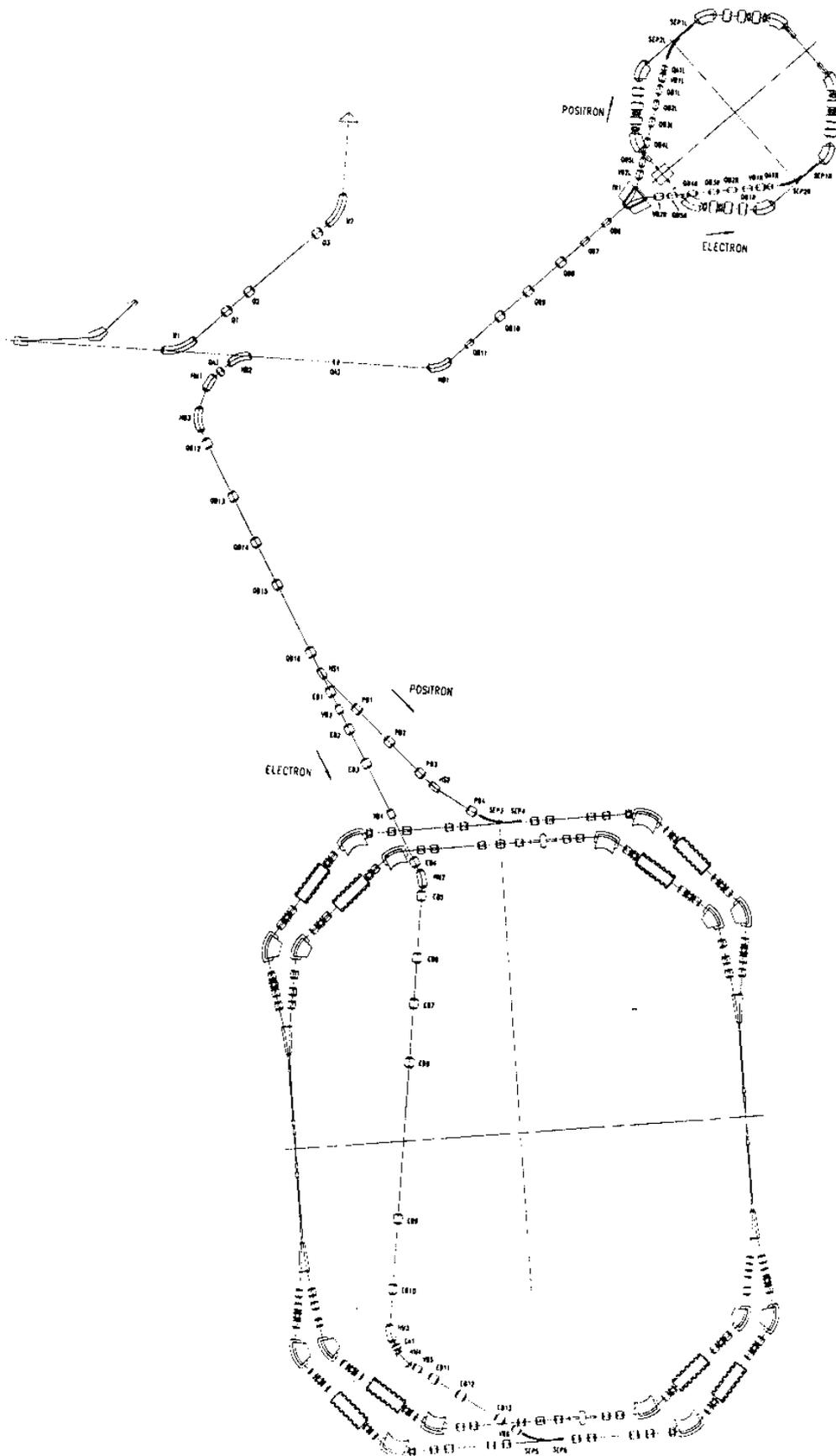
*Fig. 1-a: The lay-out of the DAΦNE transport lines with the accumulator ring and the main rings.*
