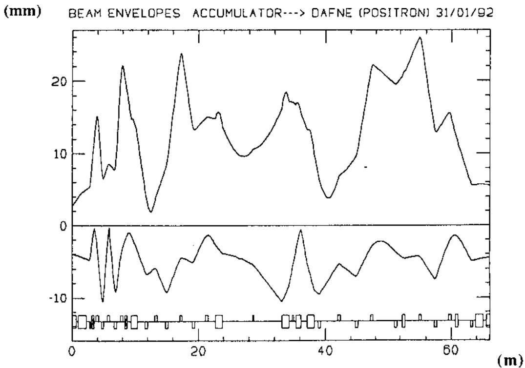
Fig. 4-b: The horizontal and vertical beam-envelope as a function of distance for the **positron** 'OUT' beam. The beam-emittance for each plane is  $3 \times 10^{-7} \text{m.rad.}$ .
