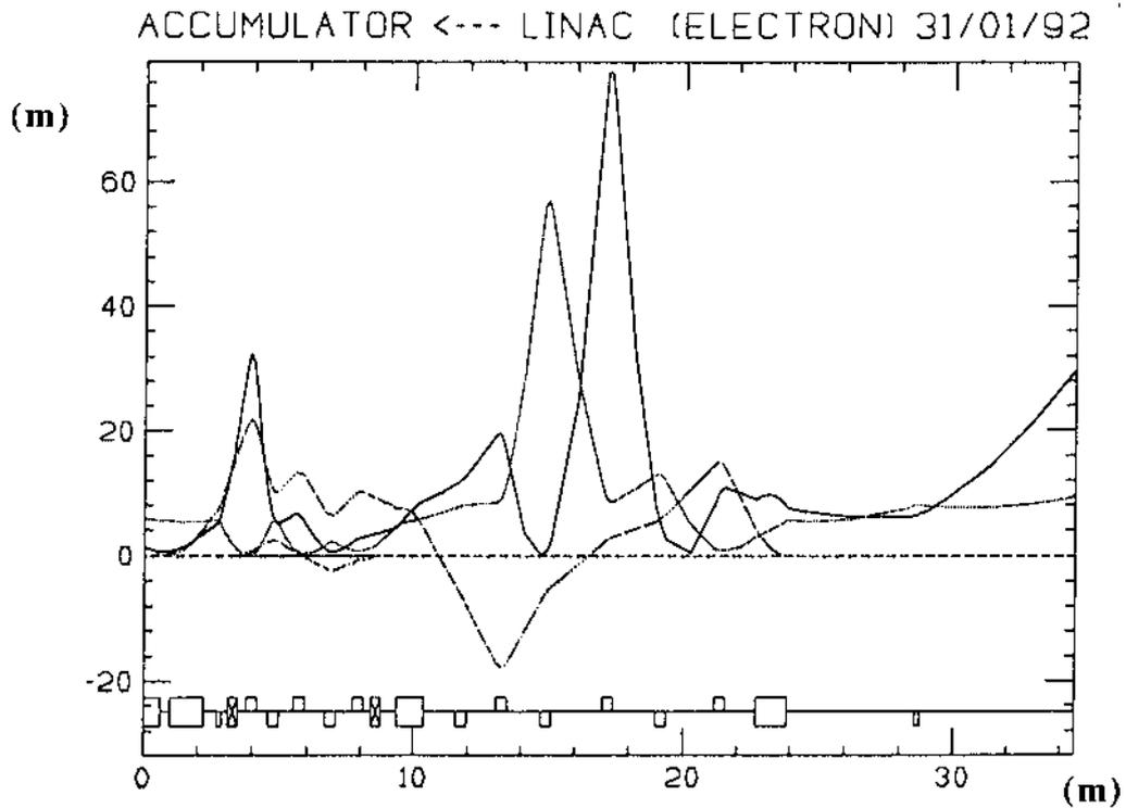
Fig. 3-a: The optical functions of **electron** 'IN' beam to the accumulator (the left side).
