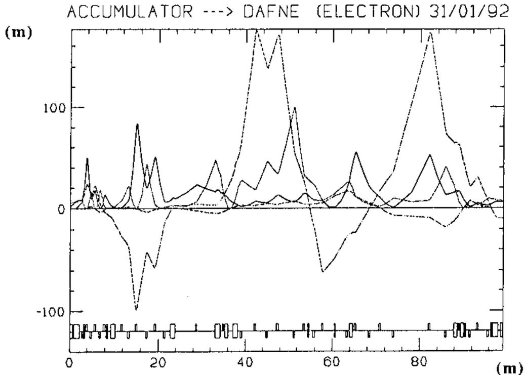
*Fig. 5-a: The optical functions of **electron** 'OUT' beam from the accumulator (the left side) to one of the main rings (to the right) through the short branch. The solid line corresponds to  $\beta_x$  and the dotted line to  $\beta_z$ . The dot-dashed line represents ten times the horizontal dispersion ( $10 \eta_x$ ) and dashed line is ten times vertical dispersion ( $10 \eta_z$ ).*
