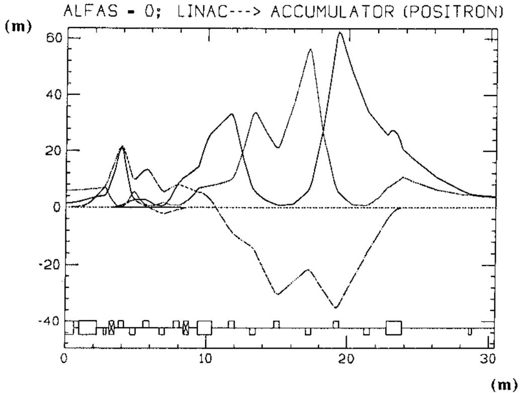
Fig. 6-a: The optical functions of a fictitious ring for **positron** 'IN' solution with  $\alpha_i = 0$ ,  $\eta_i$ ,  $\eta'_i = 0$ . The drift space at the right most end has been slightly shortened to obtain the reflective symmetry.
