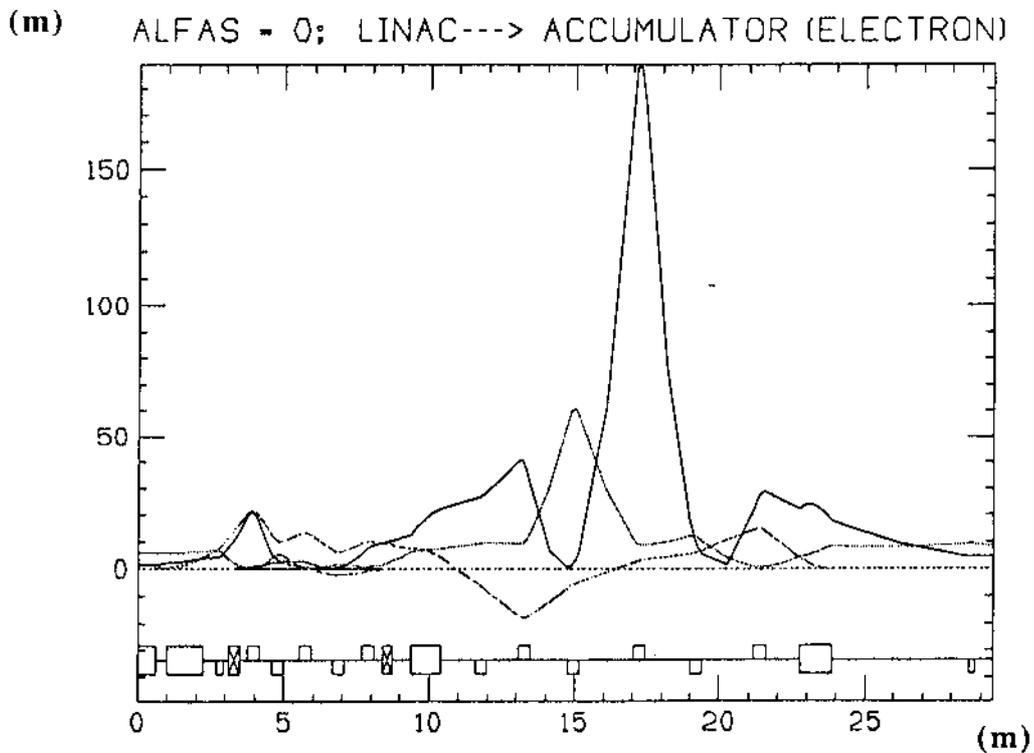
Fig. 6-b: The optical functions of a fictitious ring for **electron** 'IN' solution with  $\alpha_i = 0$ ,  $\eta_i$ ,  $\eta'_i = 0$ . The drift space at the right most end has been slightly shortened to obtain the reflective symmetry.
