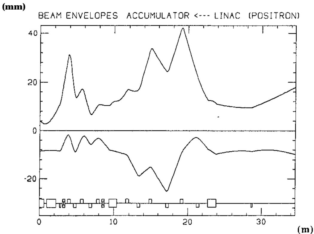
**Fig. 2-b:** The horizontal and vertical beam-envelope as a function of distance for the **positron** 'IN' beam. The beam-emittance for each plane is  $1.0 \times 10^{-5}$  m.rad..
