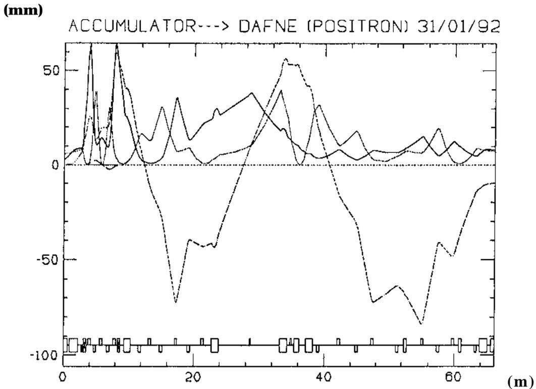
Fig. 4-a: The optical functions of **positron** 'OUT' beam from the accumulator (the left side) to one of the main rings (to the right) through the short branch. The solid line corresponds to  $\beta_x$  and the dotted line to  $\beta_z$ . The dot-dashed line represents ten times the horizontal dispersion ( $10 \eta_x$ ) and dashed line is ten times vertical dispersion ( $10 \eta_z$ ).
