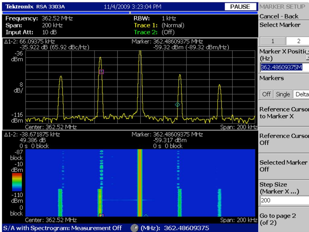
Fig. 3 – Positron beam longitudinal behavior shows “in collision – out of collision” case.
