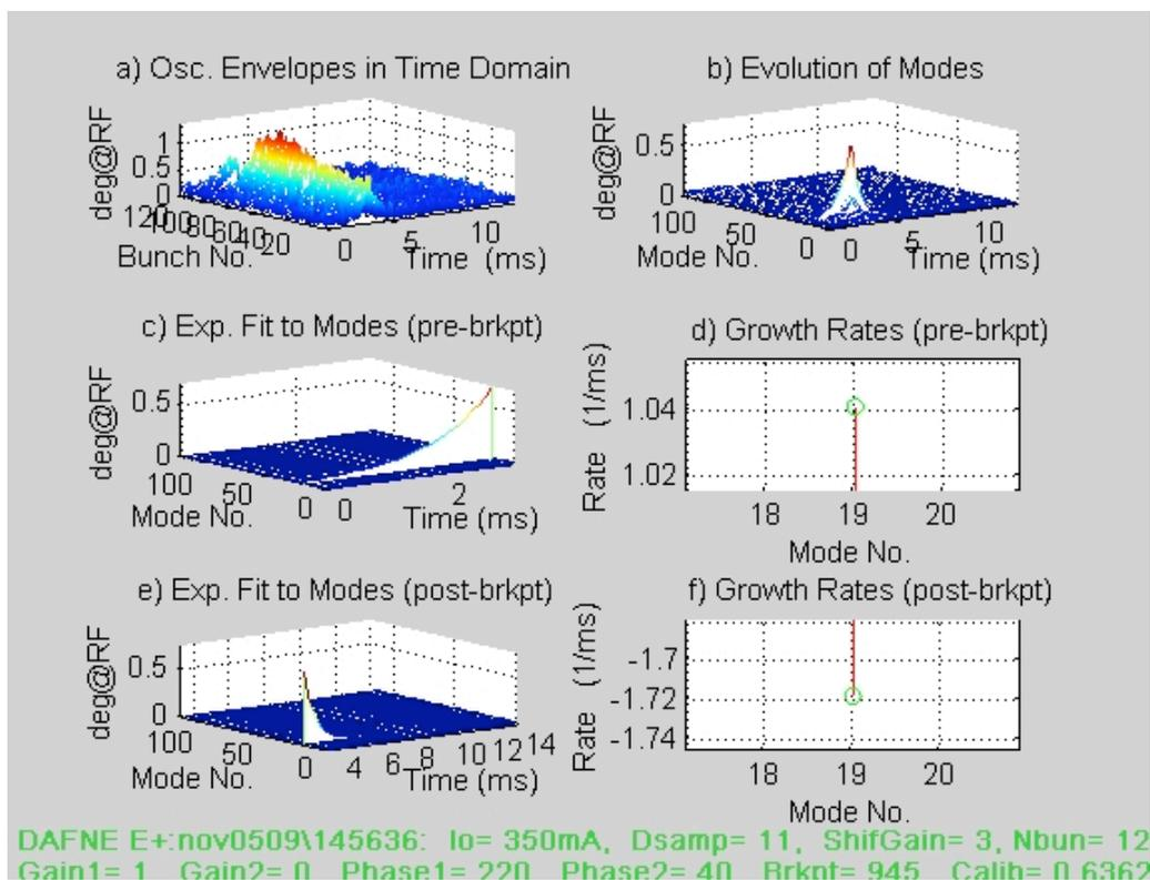
Fig. 11 – The Modal growth rate in collision is  $1.04 \text{ ms}^{-1}$ .
