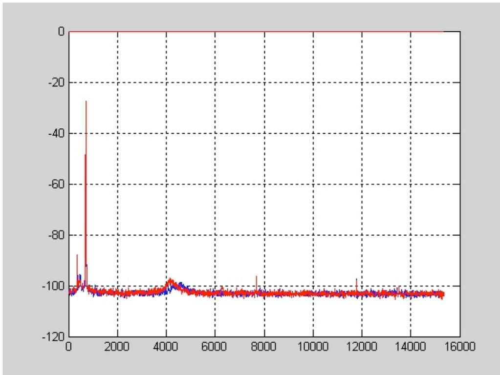
Fig. 4 – Data from the spectrum analyzer (the highest peak is the  $e^+$  118-th harmonic) elaborated by MATLAB: in red beams out of collision, in blue beams in collision. The vertical scale is in dBm, the horizontal scale shows the number of bin (frequency).
