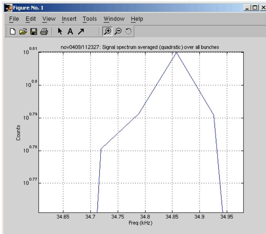
Fig. 12 – The Synchrotron frequency (out of collision) is 34.86 kHz.
