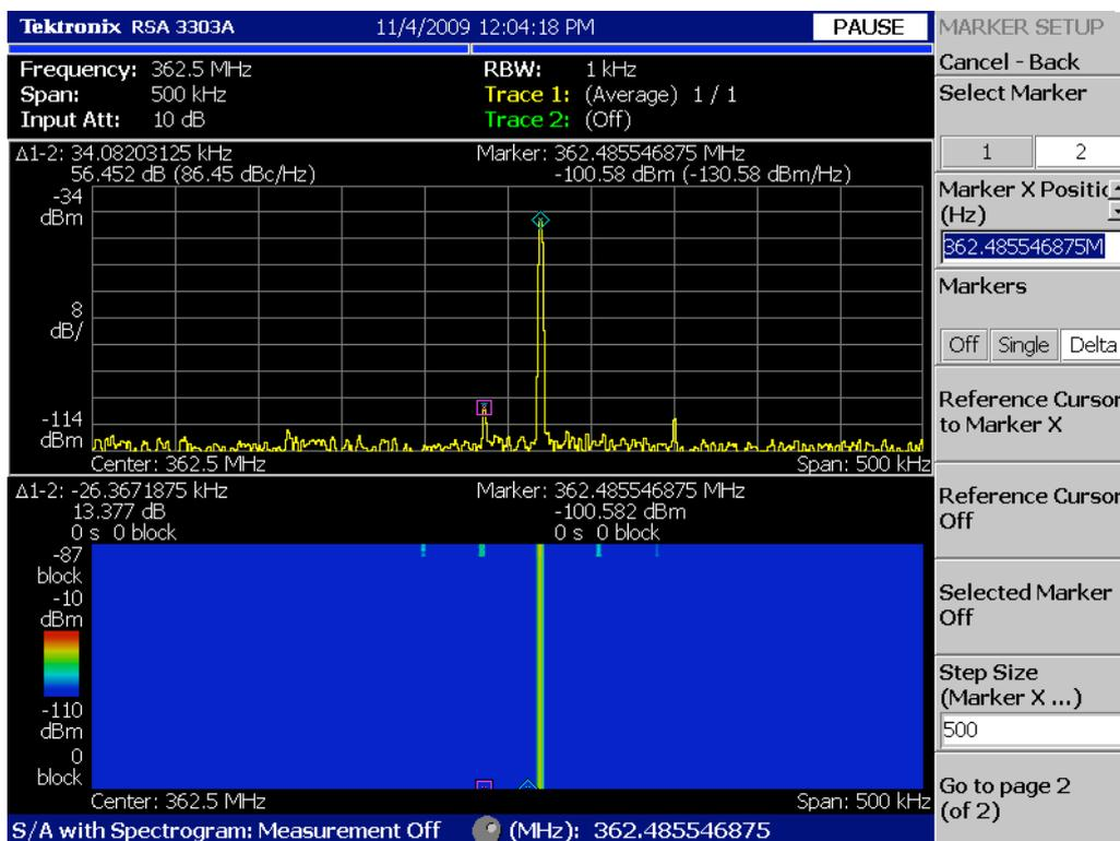
Fig. 2 – Synchrotron sidebands damped by beam-beam collisions.
