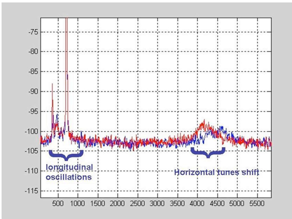
Fig. 5 – Zoom of the previous figure, showing the longitudinal and horizontal tunes.
