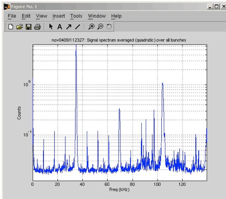
Fig. 8 – Feedback diagnostics: beam frequency spectrum, out of collision, feedback off.
