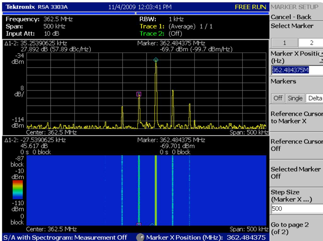
Fig. 1 – Positron 118-th RF harmonic with synchrotron sidebands.
