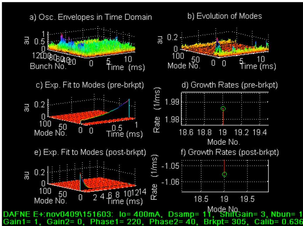
Fig. 10 – The Modal growth rate out of collision is  $1.99 \text{ ms}^{-1}$ .
