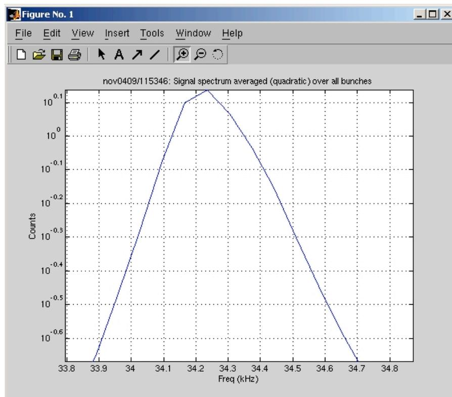
Fig. 13 – The Synchrotron frequency (in collision) is 34.23 kHz.
