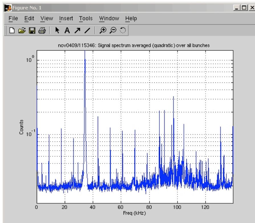
Fig. 9 – Feedback diagnostics: beam frequency spectrum, in collision, feedback off.
