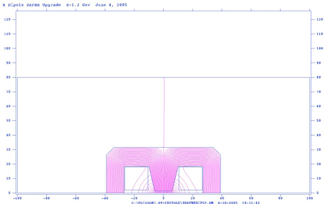
Figure 5 – 1.8 T Dipole Magnet, POISSON simulation output.
