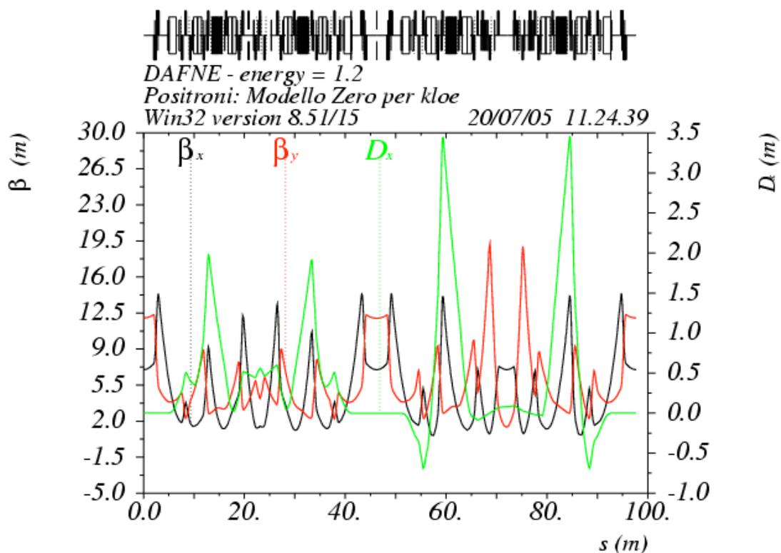
Figure 5 – Betatron and dispersion functions for DAΦNE at 1.2 GeV
