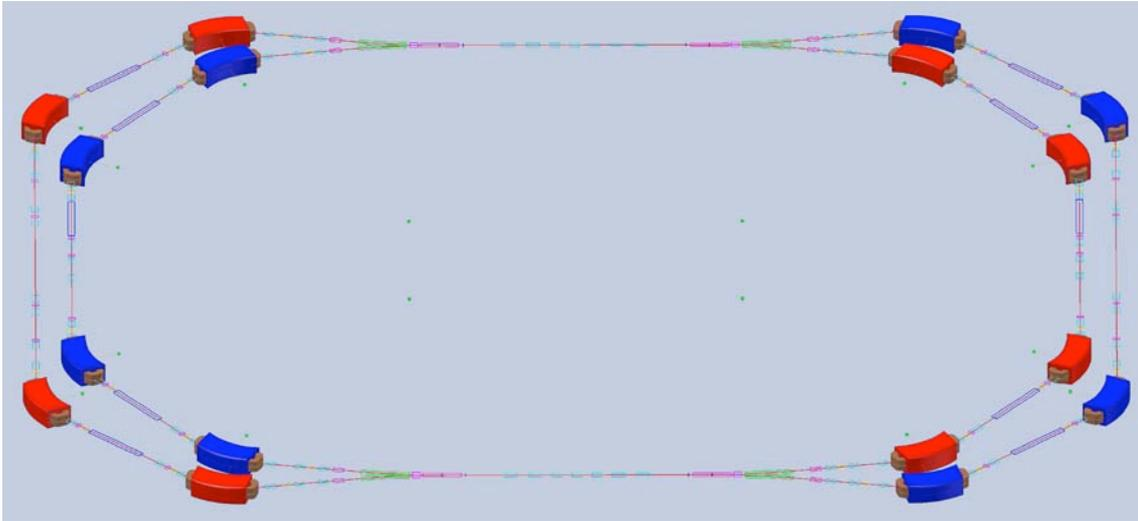
Figure 9 – Preliminary check of the transverse dipole dimensions compatibility with the present DAΦNE layout.
