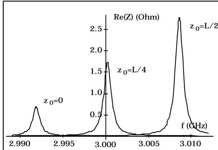
FIG. 2. Real part of the longitudinal impedance for three values of  $z_0$  ( $L=50$  mm,  $d=24$  mm,  $b=20$  mm,  $R=4$  mm,  $Q_1=2900$ ).
