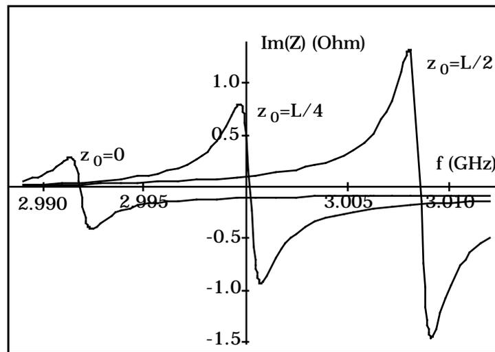
FIG. 3. Imaginary part of the longitudinal impedance for three values of  $z_0$  ( $L=50$  mm,  $d=24$  mm,  $b=20$  mm,  $R=4$  mm,  $Q_1=2900$ ).
