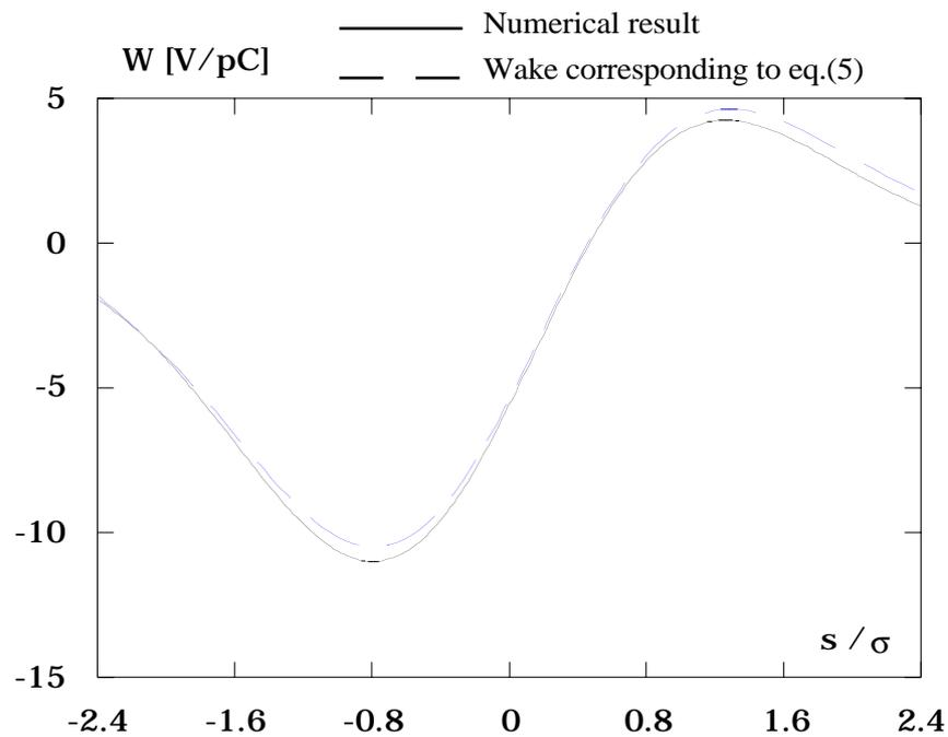
Fig. 2 - DAΦNE total wake function at  $\sigma=0.5$  cm.
