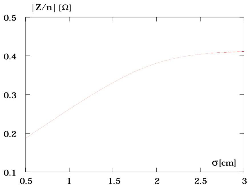
*Fig. 5 - Normalized broad-band impedance versus bunch length.*
