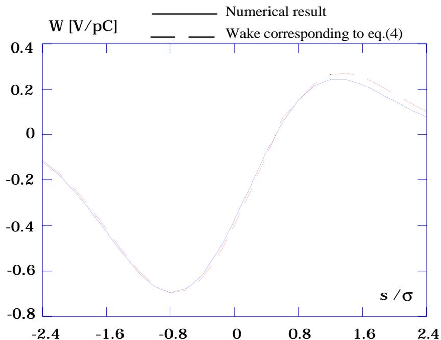
Fig. 1 - DAΦNE total wake function at  $\sigma=3$  cm.
