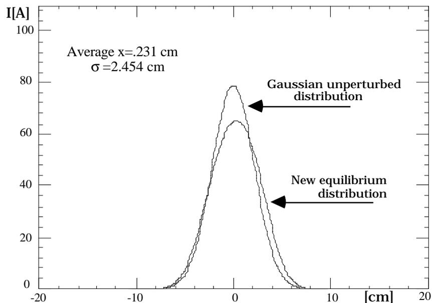
Fig. 9 - Line density distribution with an impedance double of that estimated and  $V_{RF} = 254$  KV.
