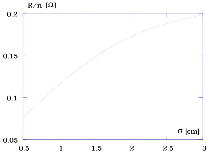
*Fig. 4 - Resistive part of DAΦNE normalized impedance.*
