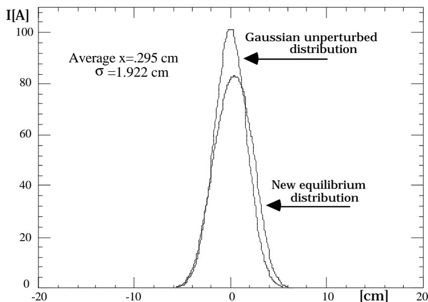
Fig. 7 - Line density distribution for  $V_{RF} = 254$  KV.
