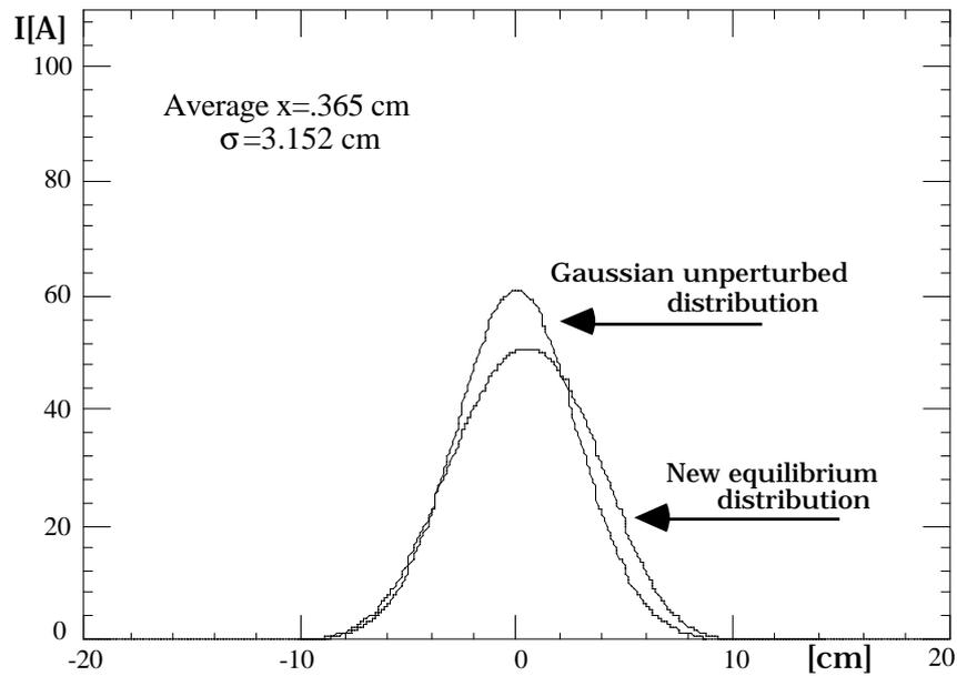
Fig. 10 - Line density distribution with an impedance double of that estimated and  $V_{RF} = 127$  KV.
