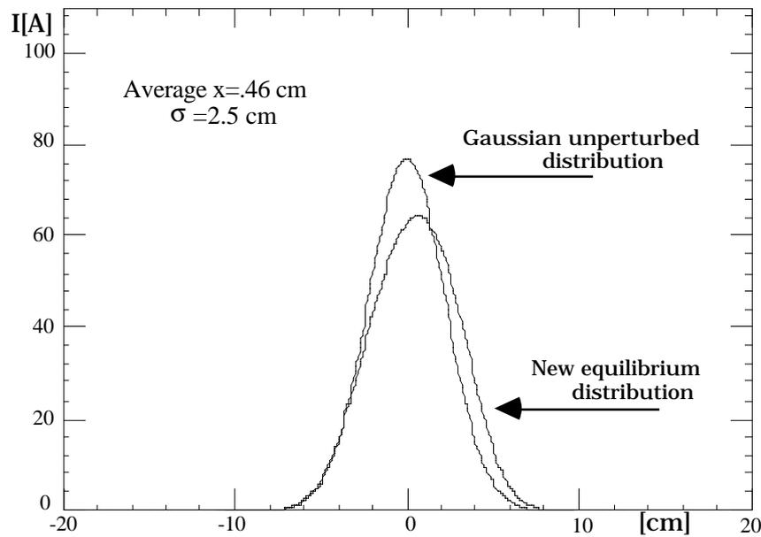
Fig. 8 - Line density distribution for  $V_{RF} = 127$  KV.
