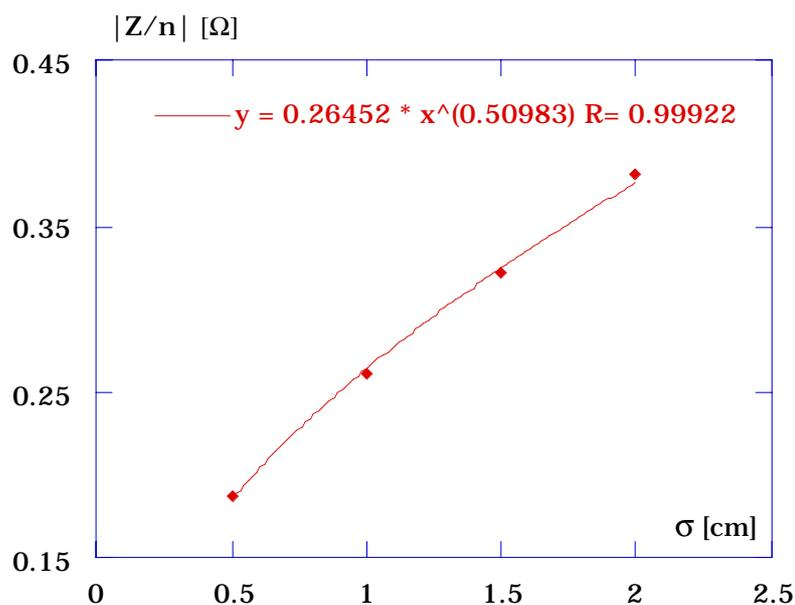
Fig. 6 - Fit of the normalized impedance versus bunch length.
