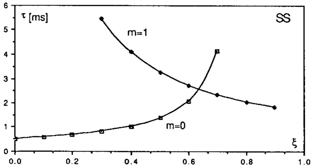
Fig. 3 - Rise times of the resistive wall instability for modes  $m=0$  and  $m=1$  in the DAΦNE accumulator for stainless steel vacuum chamber ( $\nu_x = 2.89$ ,  $\nu_y = 0.91$ ) versus chromaticity.
