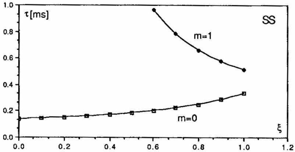
Fig. 4a) - Rise times for modes  $m=0$  and  $m=1$  with the coupled=bunch mode number  $s=25$  in the DAΦNE main ring (for stainless steel vacuum chamber) versus chromaticity.
