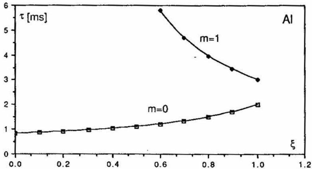
Fig. 4b) - Rise times for modes  $m=0$  and  $m=1$  with the coupled=bunch mode number  $s=25$  in the DAΦNE main ring versus chromaticity - the case of aluminium vacuum chamber.
