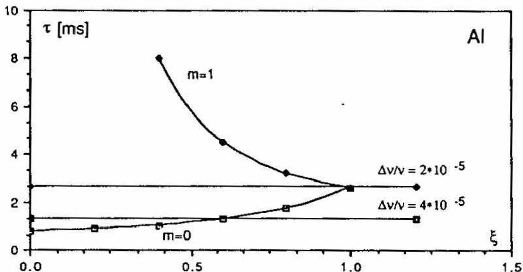
Fig. 5- Results of instability rise time calculation with BBI code for modes  $m=0$  and  $m=1$  for the DAΦNE main ring (for Al). Straight lines correspond to Landau damping time due to octupole - introduced tune spread  $\Delta v/v$ .
