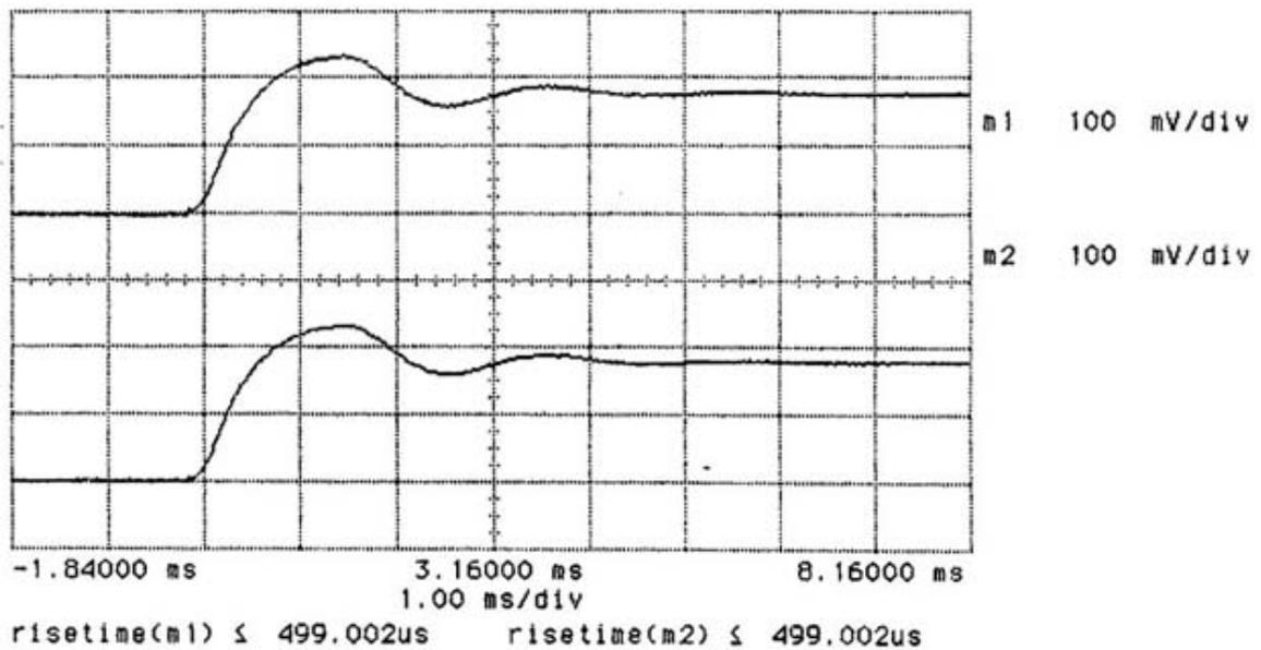
**Figure 10. Rise time. Upper one: without chamber; lower one: with chamber.**
