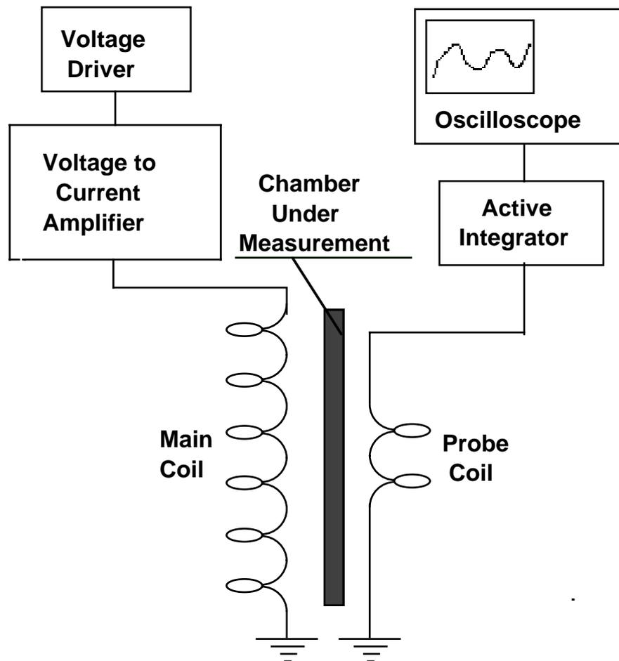
**Figure 2. Measurement Set-up.**
