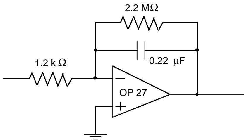
**Figure 3. Active Integrator Circuit.**
