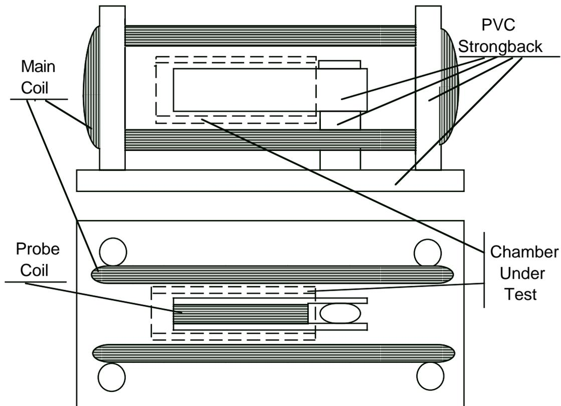
**Figure 1. Two Coil System.**
